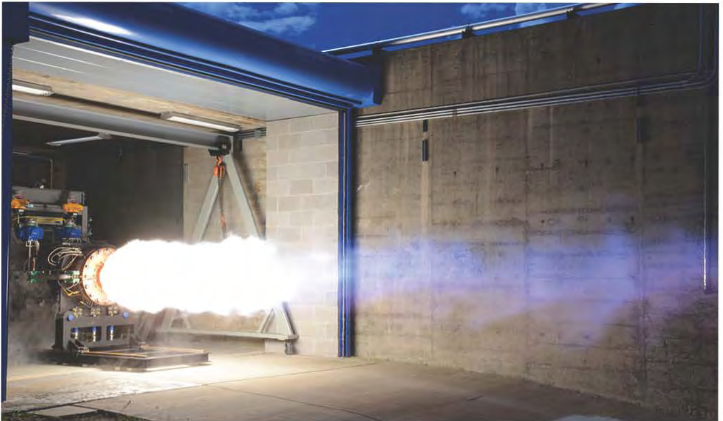
Figure 4-10. ORBITEC's 30,000 Pound Thrust Vortex Engine
