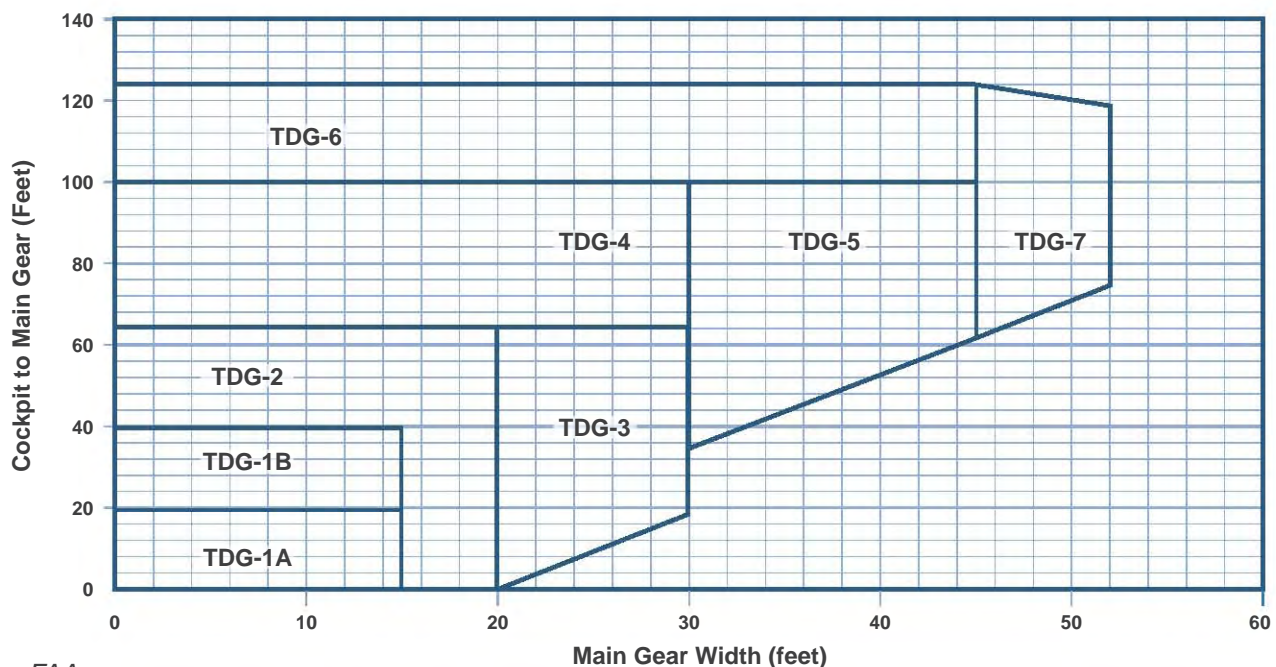
Figure 4-1. Taxiway Design Groups (Figure 1-1 from AC 150/5300-13A)
