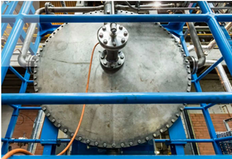
Figure 12 – Post-Combustion Carbon Capture – Amine solvent with Rotating Packed Beds (Carbon Clean)
