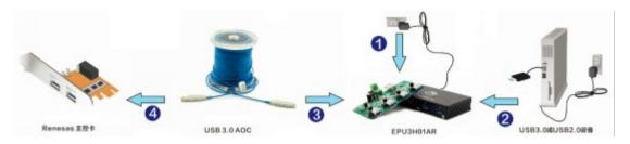
Step one: Connect the power adapter to EPU3H01AR.
