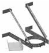
Chimney/Tee Support (Adj 8"-15") 6DT-XWS (Supports up to 20' of chimney)
