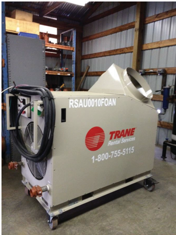
Figure 7. RSAU0010F1 (2 supply style AHU)
