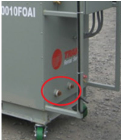
Figure 36. RSAU0010F0 - Victaulic water lines
