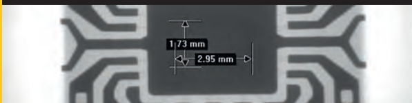
Fig 5 Suspect part close-up with die measurements
