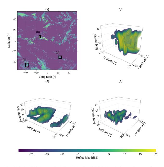
**Figure 6.** Prediction of 3D cloud structures from the Res-UNet along the FD MSG SEVIRI domain with a a top-view on the maximum cloud column reflectivity for each pixel on 06 May 2016, 13:00 UTC (a). The detailed views in (b), (c), and (d) span several tiles of 100 x 100 pixels ( $2.5^{\circ}$  on the geographic grid) to point out the absence of artifacts between predictions.
