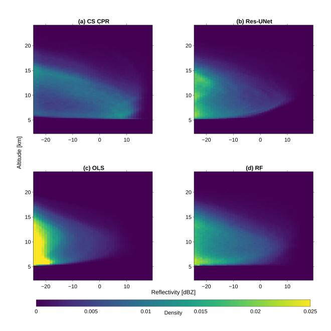
**Figure 2.** Height dependent reflectivity distribution for every height bin between 2.4-24 km for the CloudSat data (CS CPR) (**a**), the Res-UNet (**b**), the ordinary least squares model (OLS), (**c**), and the Random-Forest regression (RF) (**d**) (n = 1500).
