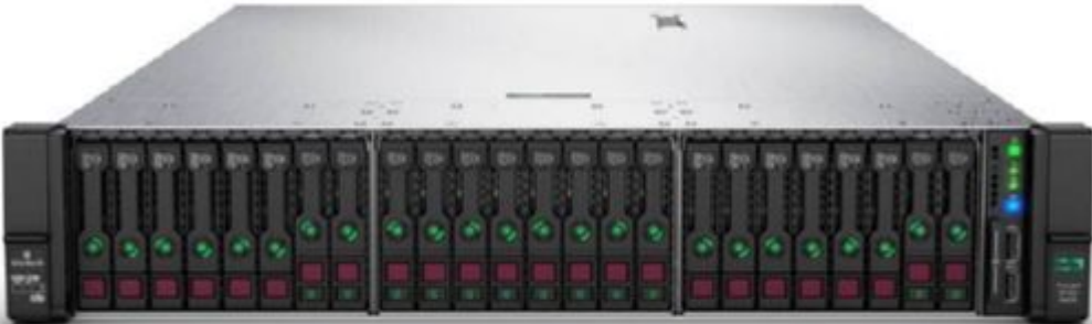
24 SFF (incl 12 NVMe SSDs) hot-plug drive model
