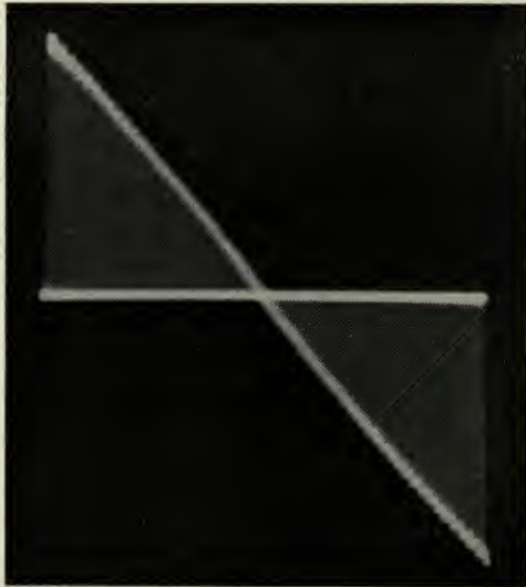
Fig. 25. Output of expander (vertical) vs. input to compressor (horizontal).
