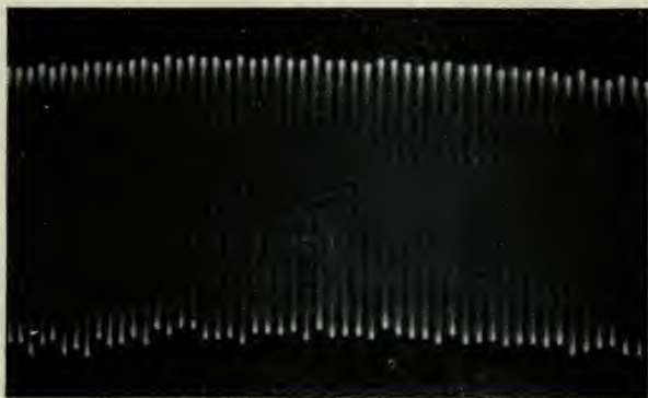
Fig. 7—Variation of quantizing current with beam deflection.
