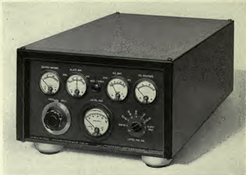
Fig. 33—Crystal chronometer for geophysical studies, consisting of 100 KC. GT-cut crystal, bridge oscillator, and frequency converters to derive precision 500-Cycle output to operate timing devices.
