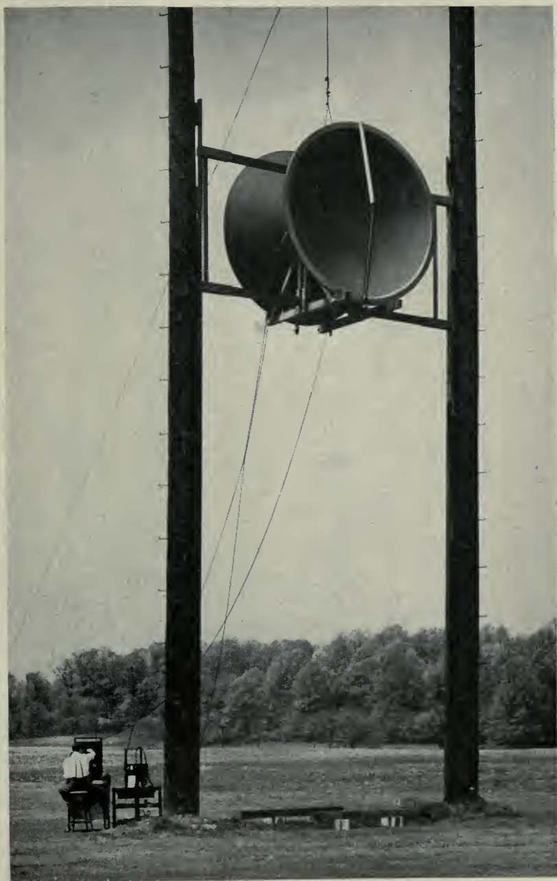
Fig. III-1.—Measuring the back to back crosstalk of two 10 ft. paraboloid antennas.
