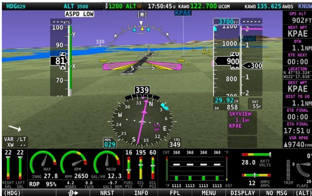
Figure 69 – SkyView HDX Synthetic Vision With Runways
