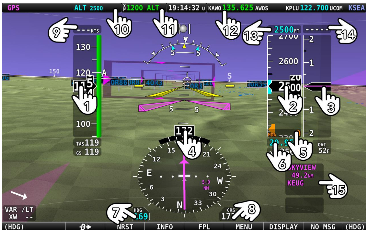
Figure 30 – Touchable on-screen regions that change Knob BUG Function; See Below for Legend
