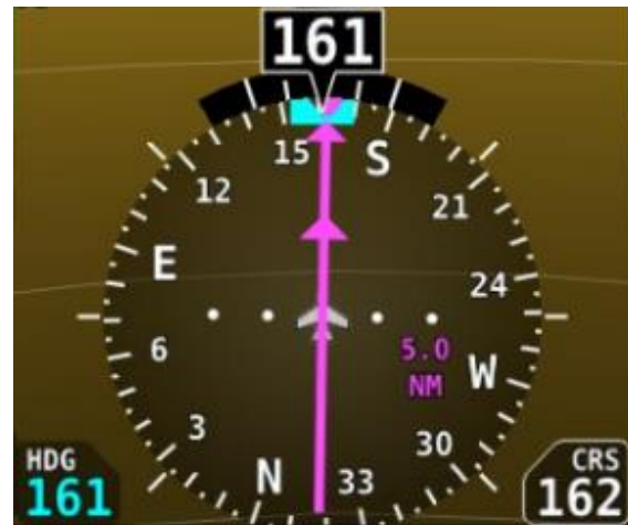
Figure 43 — HSI Example: GPS
