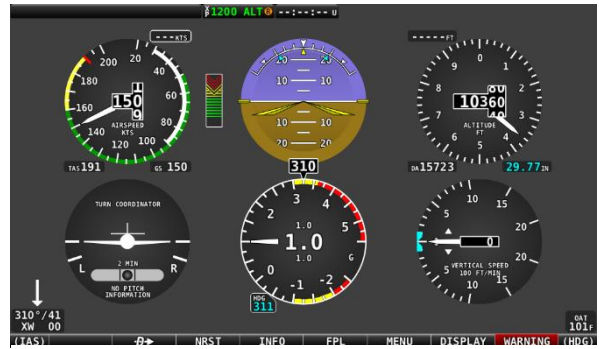
Figure 83 — G Meter in Six-Pack Presentation PFD
