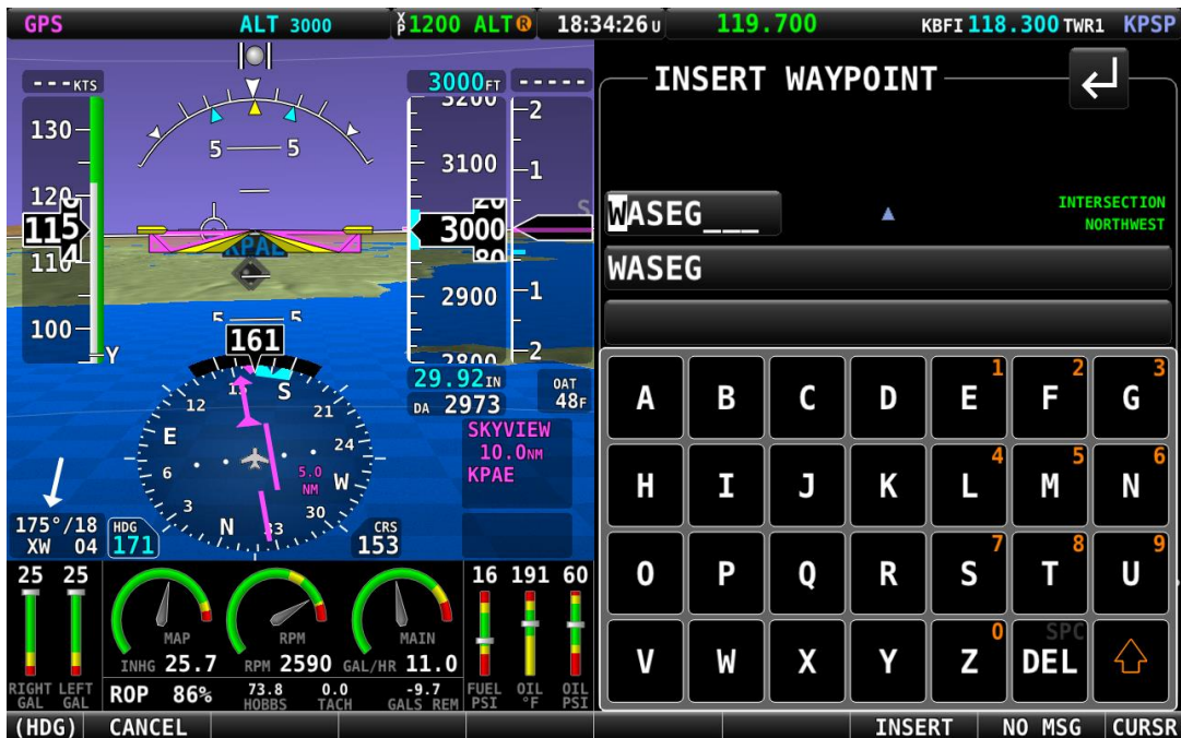
Figure 164 – Insert Waypoint Window
