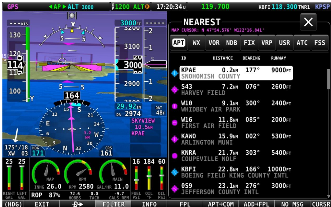
Figure 133 – Moving Map Nearest Window – Full data
