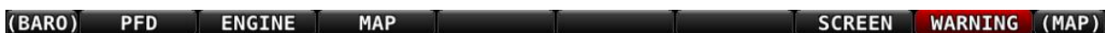
Figure 254 – Message Notification Area above button 8 (2nd from right), showing a Warning Notification
