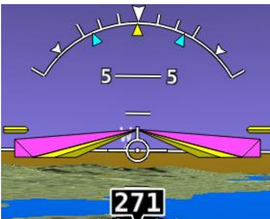
Figure 237 – Single Cue / Inverted-V with Autopilot Servos Engaged
