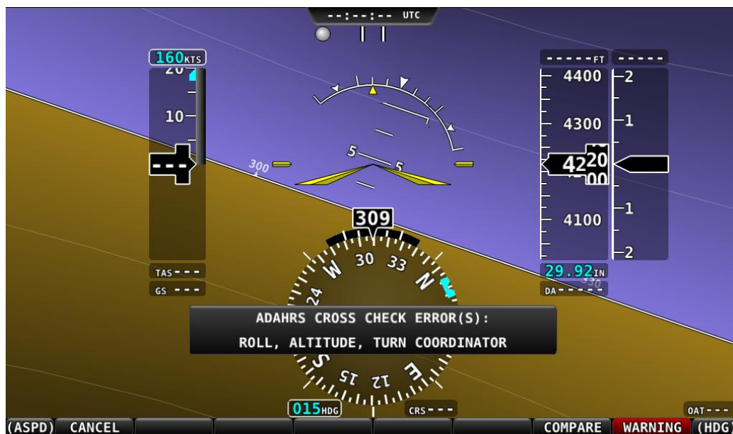
Figure 88 – ADAHRS Cross-Checking Disagreement
