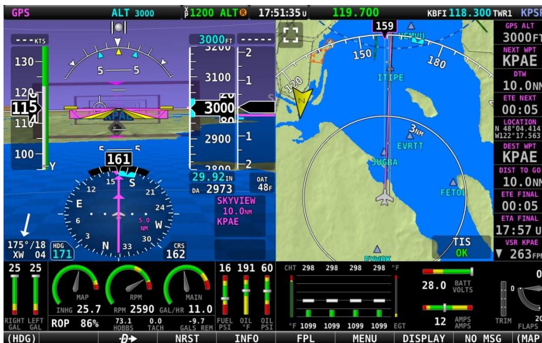
Figure 140 – Map/HSI with Navigation Active
