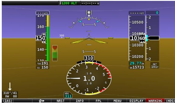
Figure 82 — G Meter in EFIS Presentation PFD
