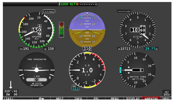
Figure 83 – G Meter in Six-Pack Presentation PFD
