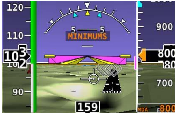
Figure 38 – MIN Bug and “MINIMUMS” Alert
