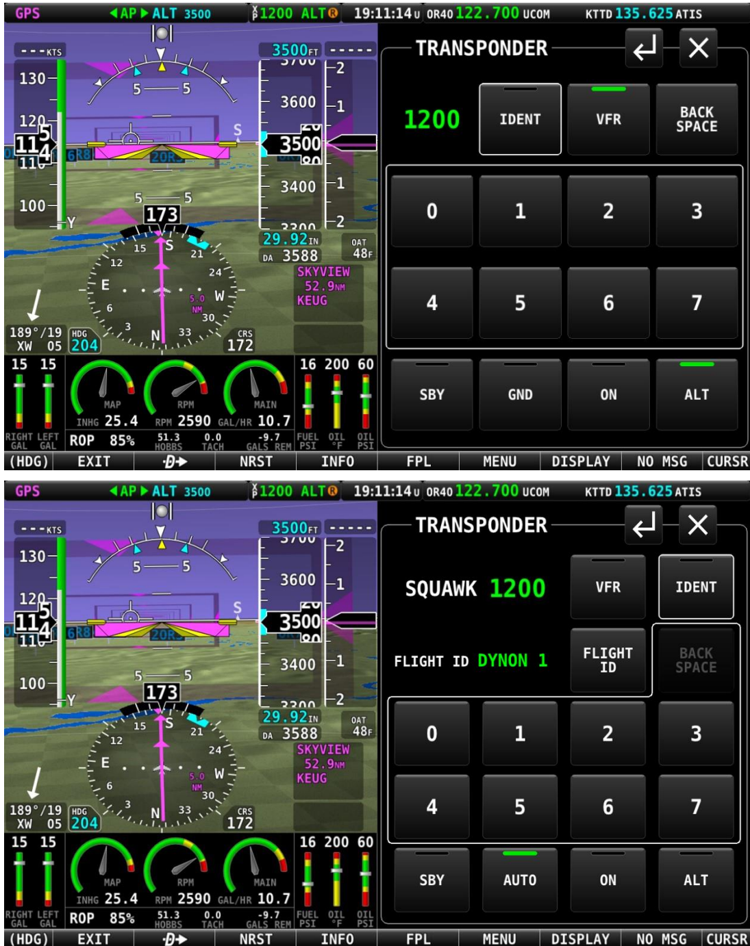
Figure 215 – TRANSPONDER control page
