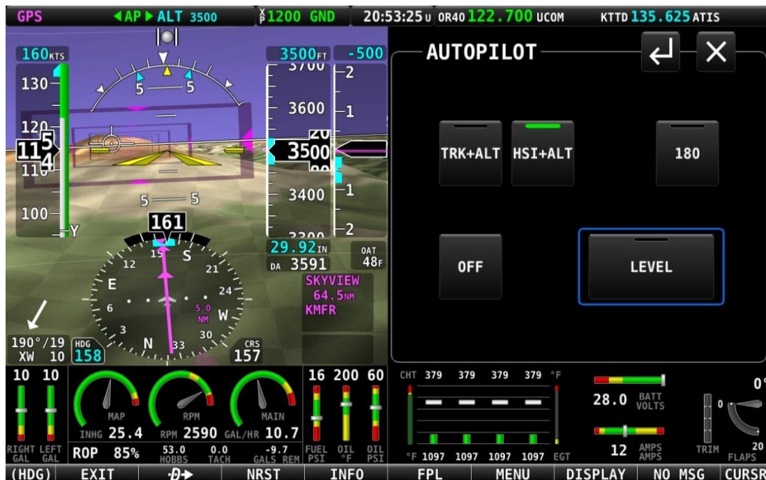
Figure 230 – HSI+ALT mode is engaged
