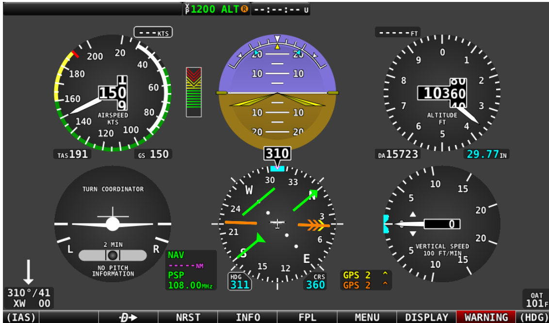
Figure 78 – Six Pack PFD Presentation, Synthetic Vision Disabled
