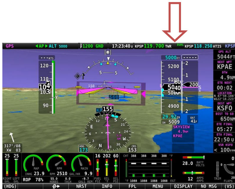
Figure 246 – SkyView Top Bar Com Radio Status Overview
