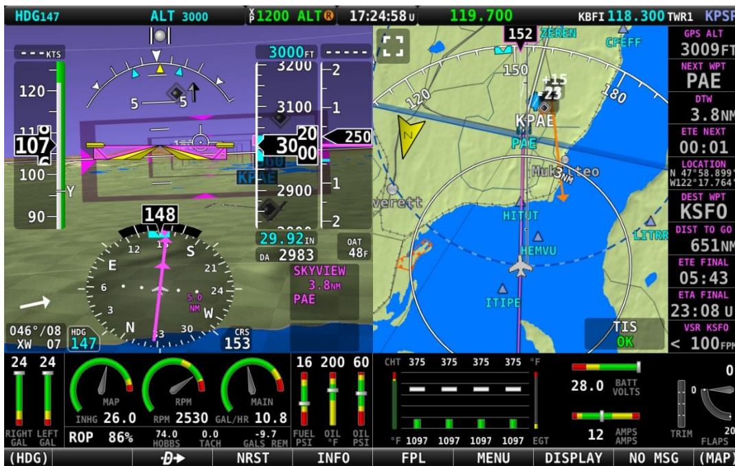
Figure 168 – Active Flight Plan: HSI and MAP Depictions
