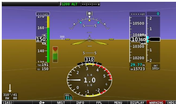
Figure 82 – G Meter in EFIS Presentation PFD
