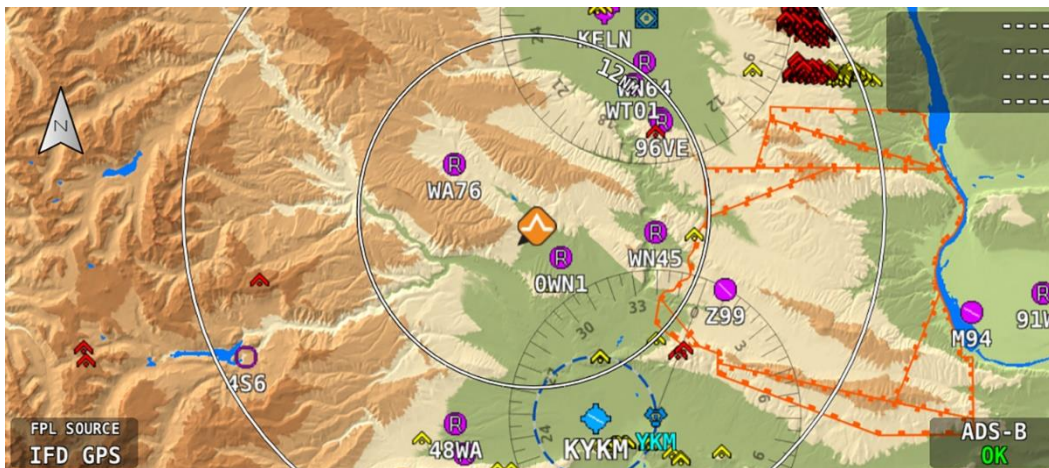
Figure 193 – Example of a PIREP Indication on Map
