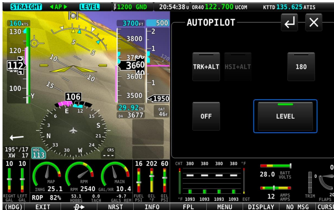
Figure 232 – LEVEL mode is engaged
