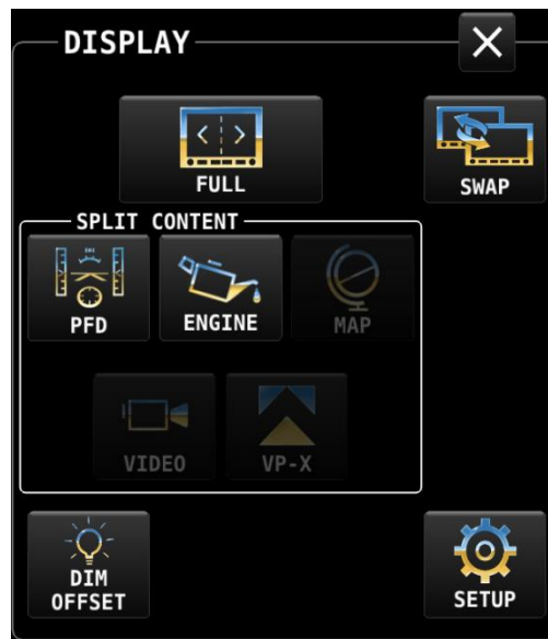
Figure 16 – DISPLAY menu showing the SWAP button
