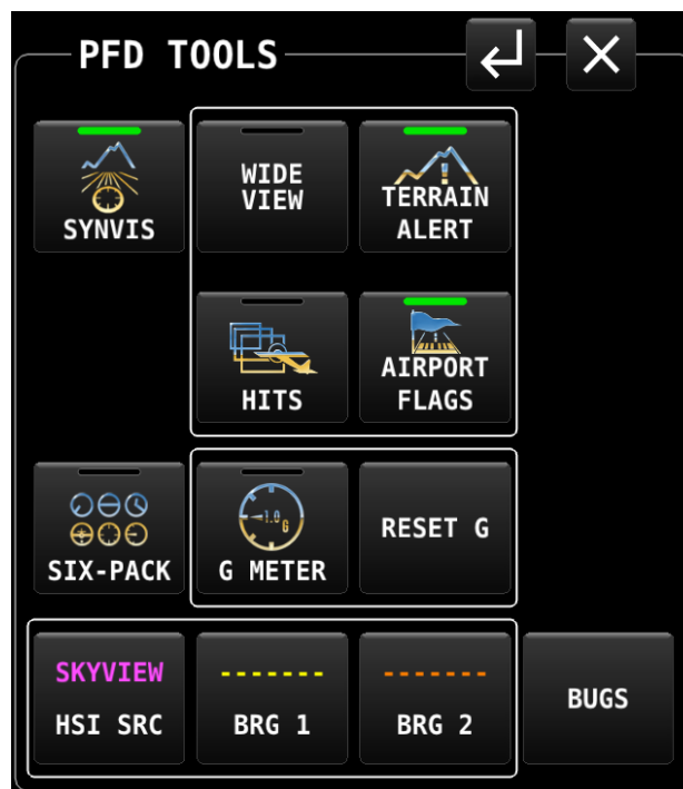
Figure 28 – PFD TOOLS menu page is shown
