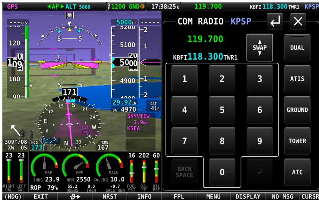
Figure 245 – Com Radio Control Panel
