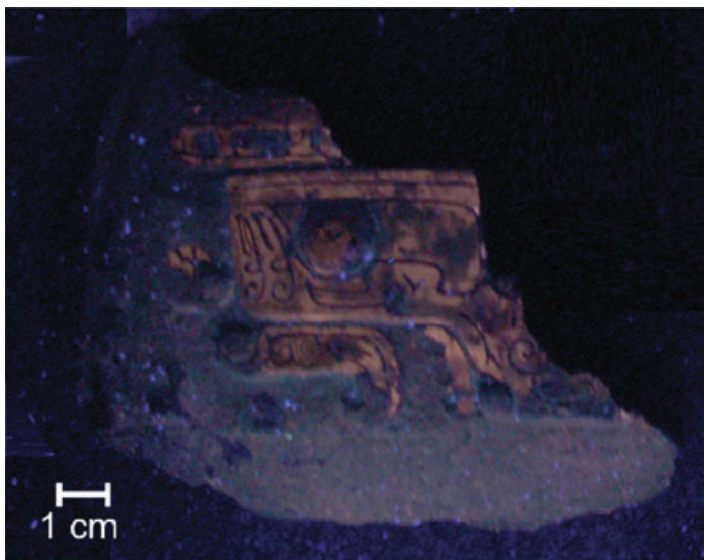
Figure 4 A photograph under ultraviolet (UV) illumination of the largest bronze fragment. Orange fluorescence, caused by the natural resin used as an adhesive for the fake corrosion, indicates the artificial patina. (Photo courtesy of S. R. Schnepf, Conservation Department, The Art Institute of Chicago; see online for a colour version.)
