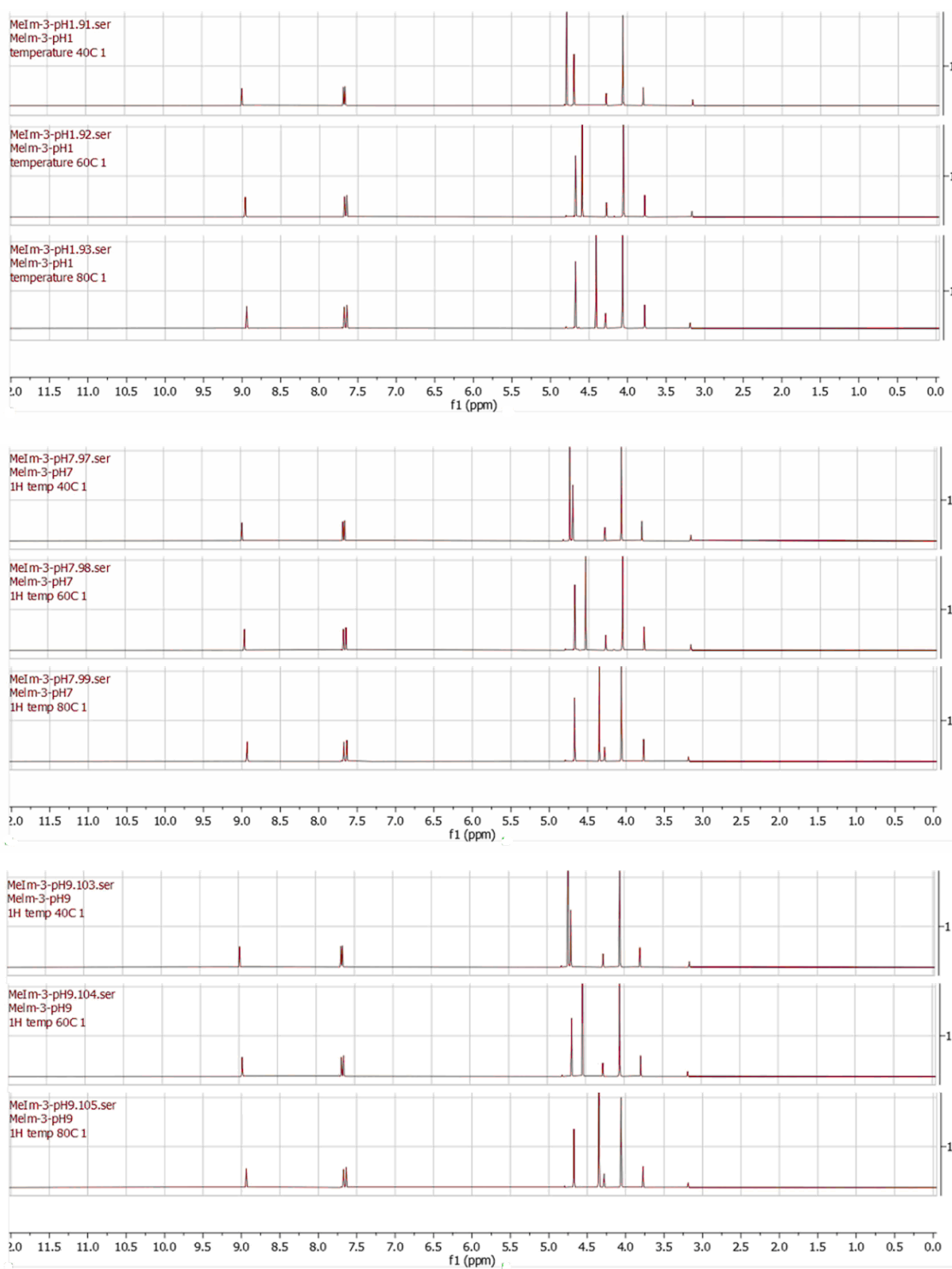
Figure 19. Thermal stability of triply charged methylimidazolium anchor Prg-O-MIM3 7 under pH 1 and temperature of 40, 60, and 80°C (upper three spectra), pH 7 and temperature of 40, 60, and 80°C (middle three spectra), and pH 9 and temperature of 40, 60, and 80°C (lower three spectra).
