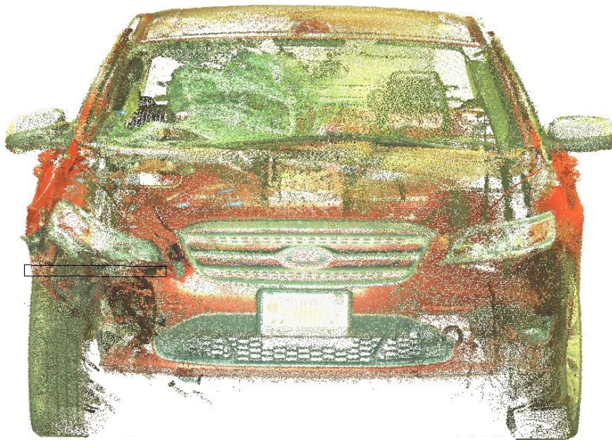
Figure 4: Front view of AG Vehicle Scan; Black rectangle is width of measurement from Figure 3.
