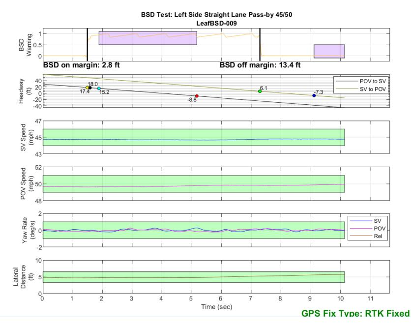
Figure D23. BSD Run 9, Straight Lane Pass-by, SV 45 mph, POV 50 mph
