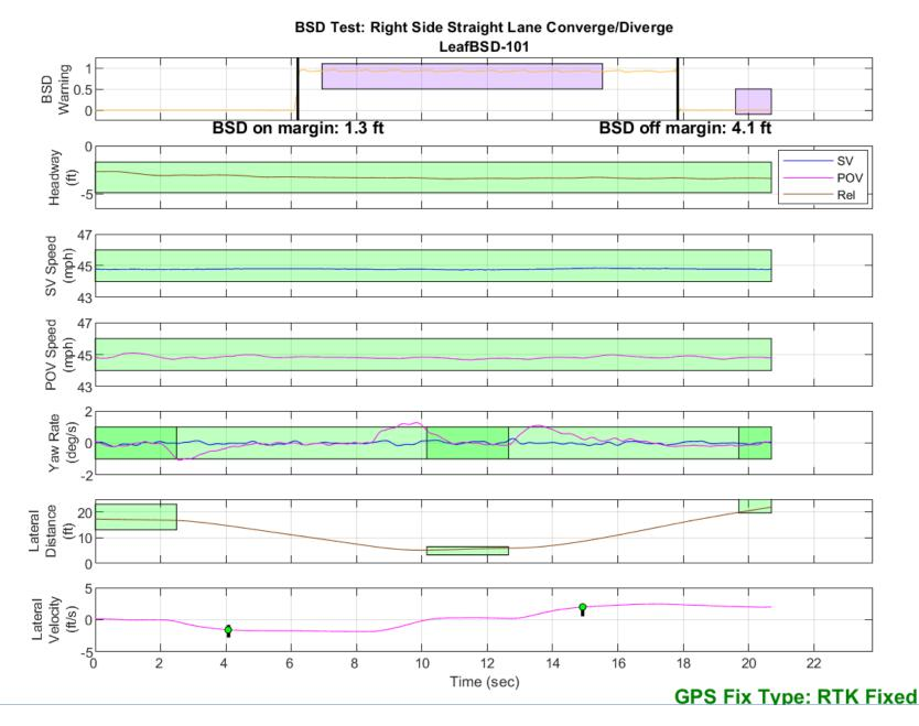
Figure D17. BSD Run 101, Straight Lane Converge/Diverge
