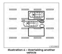
**Illustration 4:** If the driver activates the turn signal while another vehicle is in the detection zone, then the system chimes (twice) and the side indicator light flashes.
