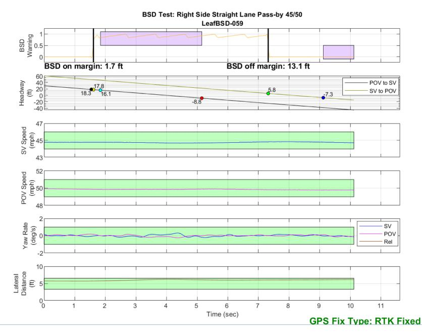
Figure D24. BSD Run 59, Straight Lane Pass-by, SV 45 mph, POV 50 mph
