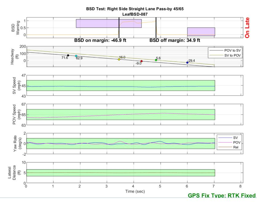
Figure D74. BSD Run 87, Straight Lane Pass-by, SV 45 mph, POV 65 mph
