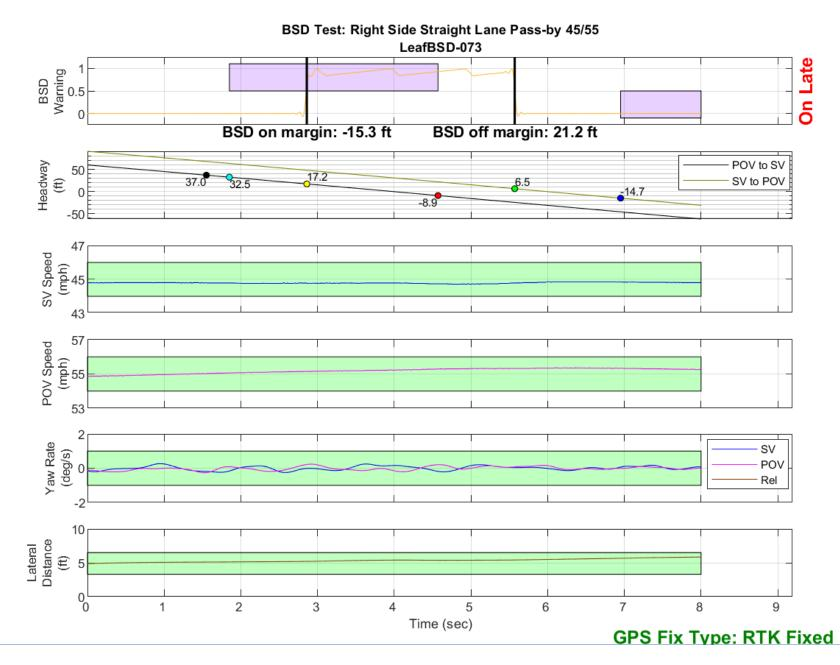
Figure D44. BSD Run 73, Straight Lane Pass-by, SV 45 mph, POV 55 mph
