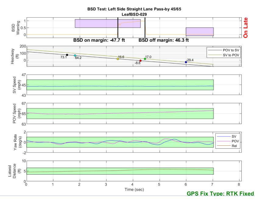
Figure D63. BSD Run 29, Straight Lane Pass-by, SV 45 mph, POV 65 mph
