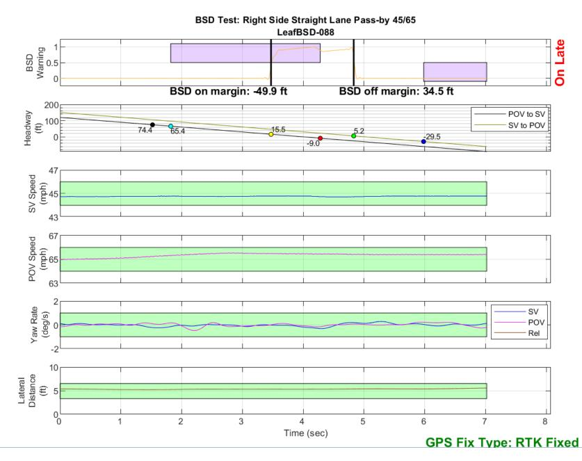
Figure D75. BSD Run 88, Straight Lane Pass-by, SV 45 mph, POV 65 mph
