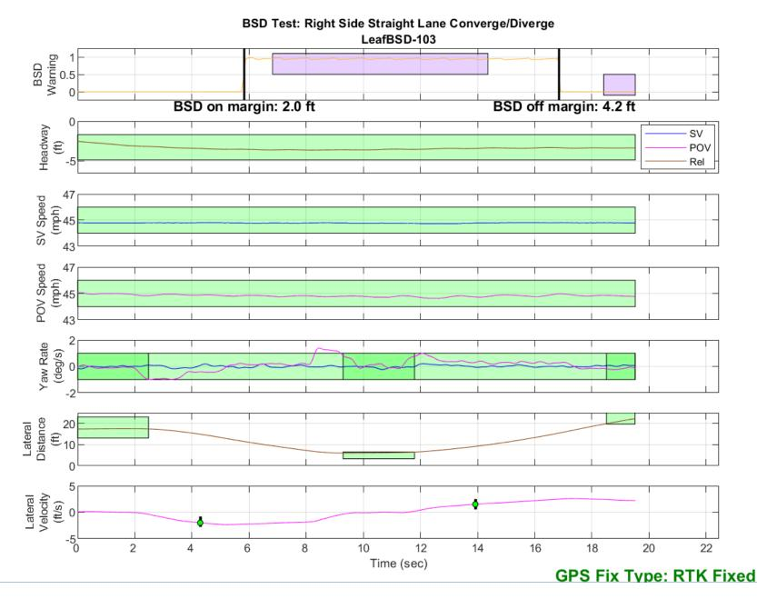
Figure D18. BSD Run 103, Straight Lane Converge/Diverge
