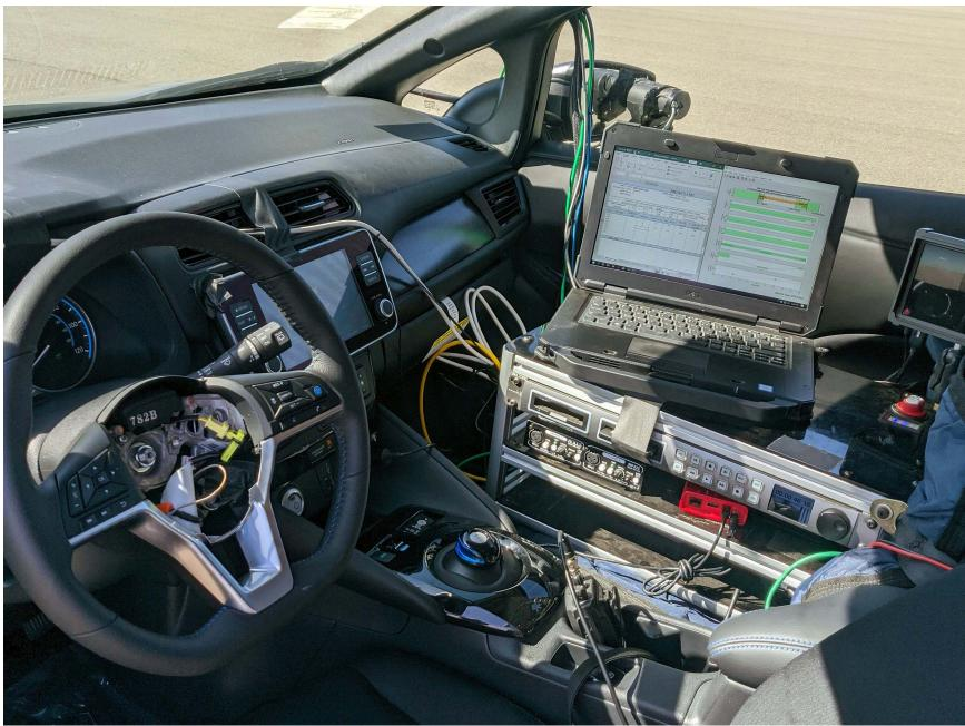
Figure A11. Computer Installed in Subject Vehicle
