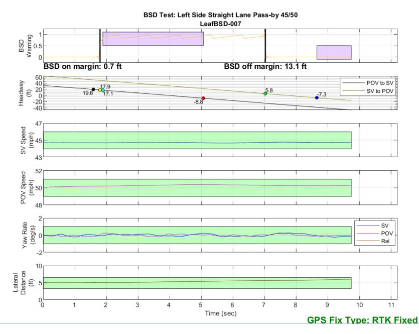
Figure D21. BSD Run 7, Straight Lane Pass-by, SV 45 mph, POV 50 mph
