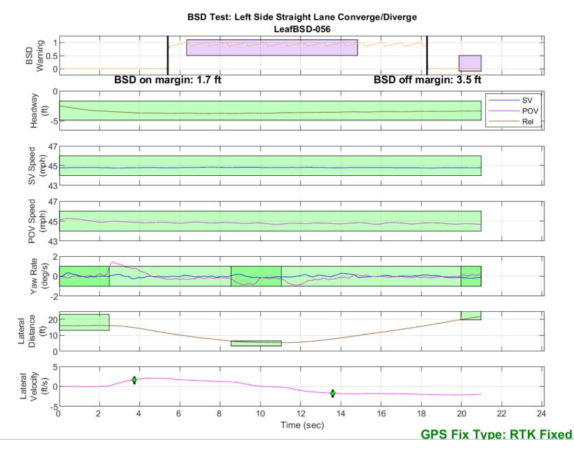
Figure D10. BSD Run 56, Straight Lane Converge/Diverge
