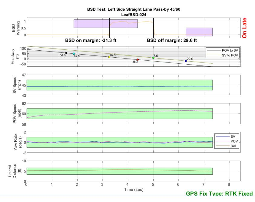
Figure D51. BSD Run 24, Straight Lane Pass-by, SV 45 mph, POV 60 mph
