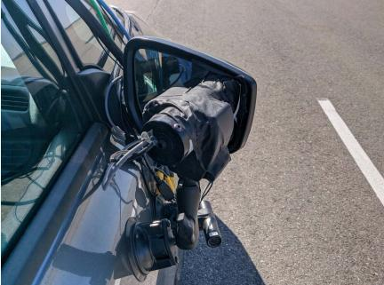
Figure A9. Sensors for Detecting Visual Alerts
