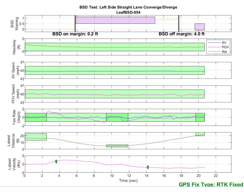
Figure D8. BSD Run 54, Straight Lane Converge/Diverge
