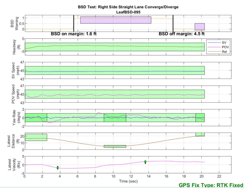
Figure D13. BSD Run 95, Straight Lane Converge/Diverge
