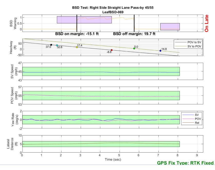
Figure D40. BSD Run 69, Straight Lane Pass-by, SV 45 mph, POV 55 mph
