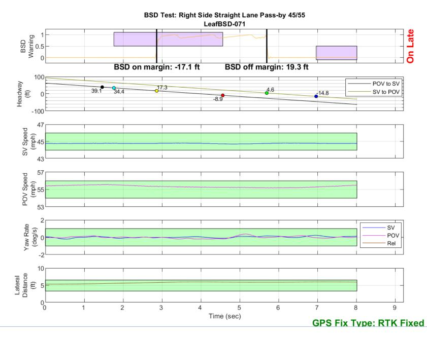
Figure D42. BSD Run 71, Straight Lane Pass-by, SV 45 mph, POV 55 mph
