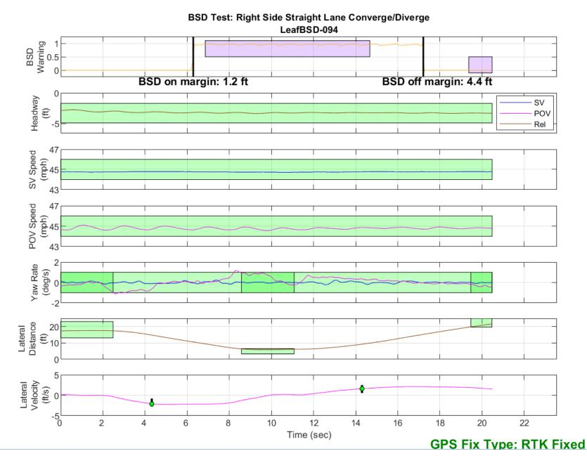
Figure D12. BSD Run 94, Straight Lane Converge/Diverge
