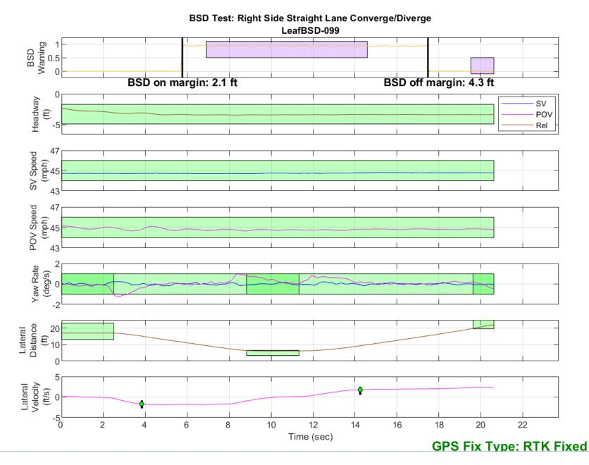
Figure D15. BSD Run 99, Straight Lane Converge/Diverge
