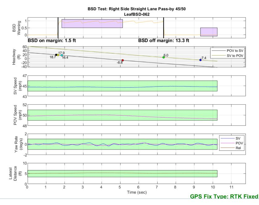
Figure D26. BSD Run 62, Straight Lane Pass-by, SV 45 mph, POV 50 mph
