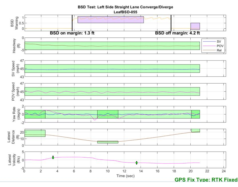
Figure D9. BSD Run 55, Straight Lane Converge/Diverge
