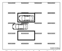
Illustration 9– Entering from the side Illustration 9: If the I-BSI system is on and your vehicle approaches the lane marker while another vehicle is in the detection zone, the system chimes (three times) and the side indicator light flashes. The I-BSI system activates to help return the vehicle back to the center of the driving lane.
