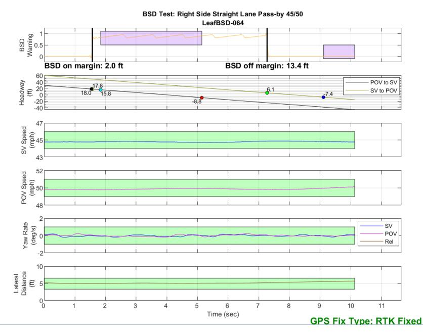
Figure D28. BSD Run 64, Straight Lane Pass-by, SV 45 mph, POV 50 mph
