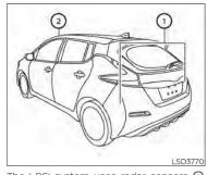
The I-BSI system uses radar sensors ① installed near the rear bumper to detect other vehicles in an adjacent lane. In addition to the radar sensors, the I-BSI system uses a camera ② installed behind the windshield to monitor the lane markers of your traveling lane.
