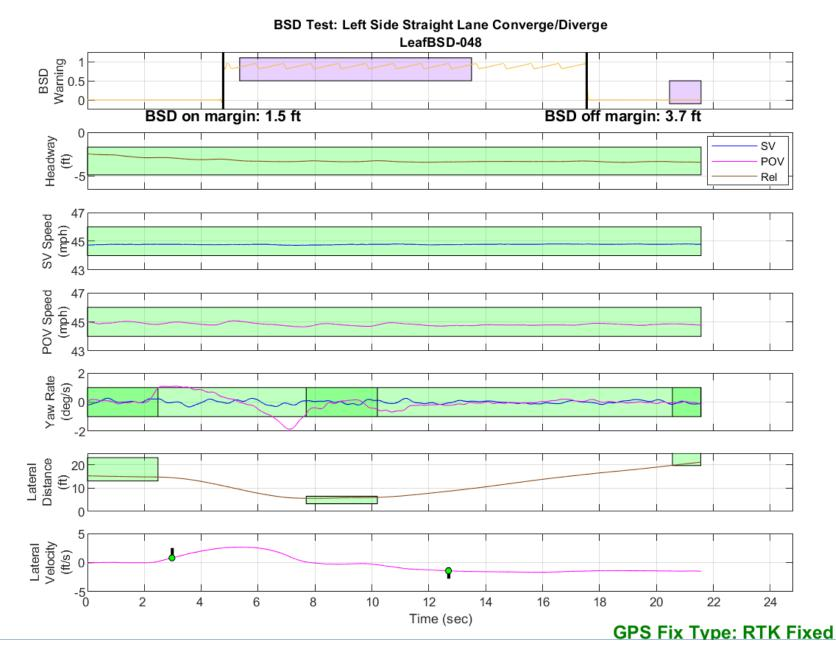
Figure D6. BSD Run 48, Straight Lane Converge/Diverge
