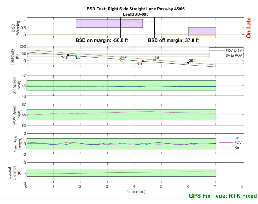
Figure D72. BSD Run 85, Straight Lane Pass-by, SV 45 mph, POV 65 mph
