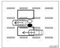
Illustration 1 – Approaching from behind BSW DRIVING SITUATIONS Illustration 1: The side indicator light illuminates if a vehicle enters the detection zone from behind in an adjacent lane.
