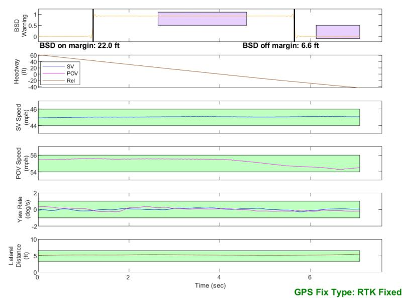
Figure D3. Example Time History for Straight Lane Pass-By Passing
