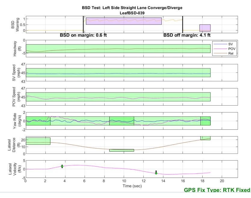
Figure D5. BSD Run 39, Straight Lane Converge/Diverge
