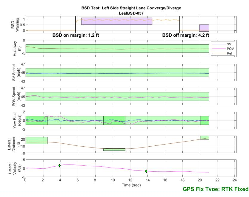
Figure D11. BSD Run 57, Straight Lane Converge/Diverge
