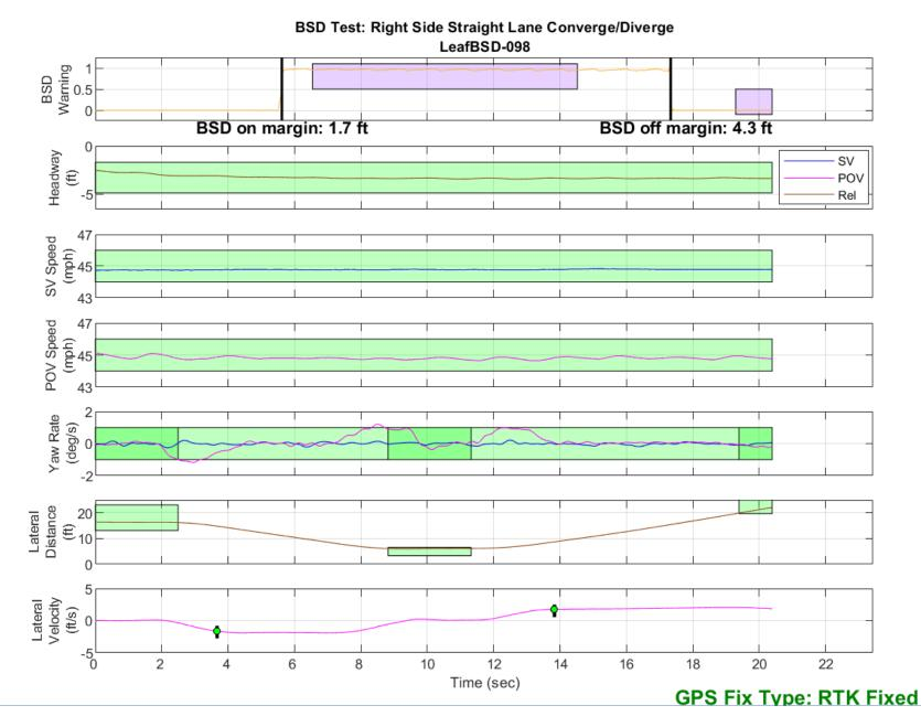
Figure D14. BSD Run 98, Straight Lane Converge/Diverge
