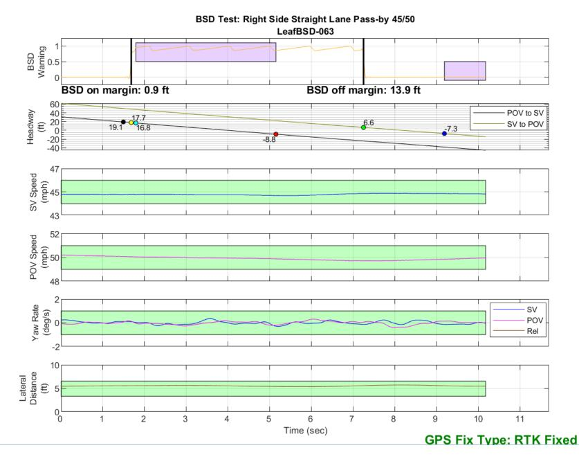
Figure D27. BSD Run 63, Straight Lane Pass-by, SV 45 mph, POV 50 mph
