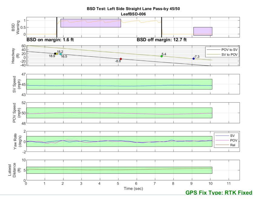
Figure D20. BSD Run 6, Straight Lane Pass-by, SV 45 mph, POV 50 mph
