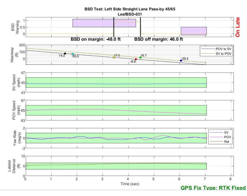
Figure D65. BSD Run 31, Straight Lane Pass-by, SV 45 mph, POV 65 mph
