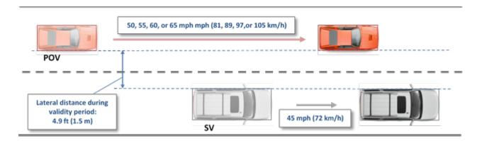
Figure 2. Straight Lane Pass-by Test (Left-side POV Pass-by is shown)
