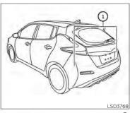
The BSW system uses radar sensors 0 installed near the rear bumper to detect other vehicles in an adjacent lane.
