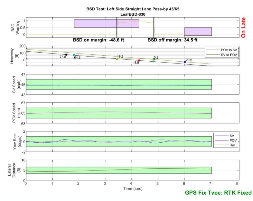
Figure D64. BSD Run 30, Straight Lane Pass-by, SV 45 mph, POV 65 mph
