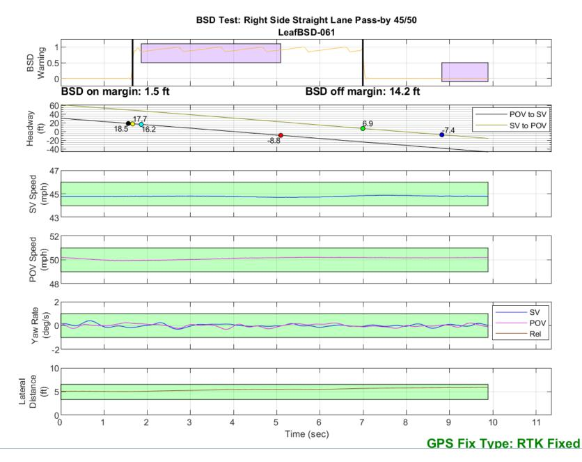
Figure D25. BSD Run 61, Straight Lane Pass-by, SV 45 mph, POV 50 mph
