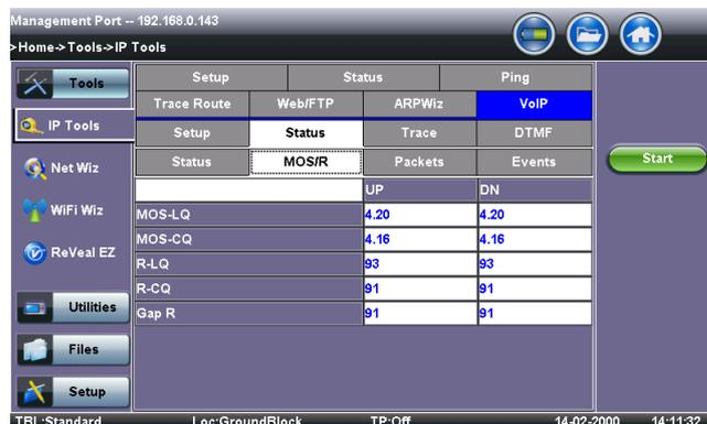
**VoIP Call Expert** – Emulates an IP phone and can place and receive calls using SIP or H.323 protocols. Comprehensive Codec support and call destination options verify voice encoding and translation provisioning. Real-time evaluation of voice quality (MOS and R-factor) is made possible using the patented Telchemy® test method.
