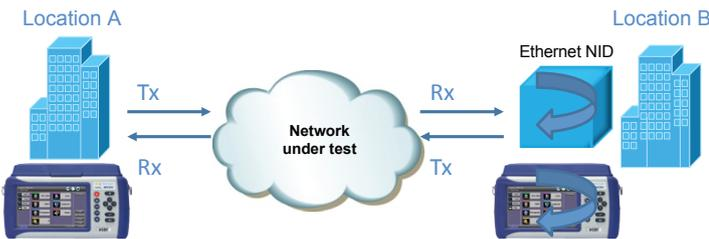
Remote Loopback to VeEX Ethernet tester or Ethernet Network Interface Device
