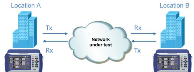
Peer to peer test: Symmetrical or Asymmetrical traffic generation Remote control from a single unit; Test results available for each direction
