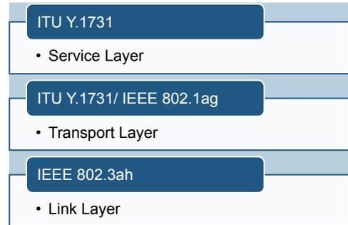
The TX300 offers a complete tool set for Link Level (IEEE 802.3ah) and Service Level (IEEE 802.1ag/ ITU- Y.1731) OAM for monitoring and maintaining carrier grade Ethernet services.
