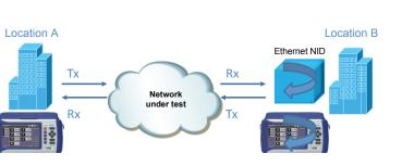
Remote Loopback to VeEX Ethernet tester or Ethernet Network Interface Device
