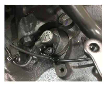
During inspection if the single gear configuration (as shown below) is found with no smaller second gear, no further action is required. Reinstall the cam position sensor.
