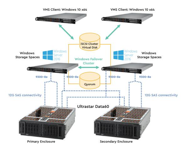
The cluster exports block storage from the iSCSI target (Ultrastar Data60) to the initiator (recording server). On the Ultrastar Data60 storage platform, it is recommended to create multiple RAID-5 volumes exposed as an iSCSI target to archive the video data. Recommended steps to create the Failover Cluster are as follows:
