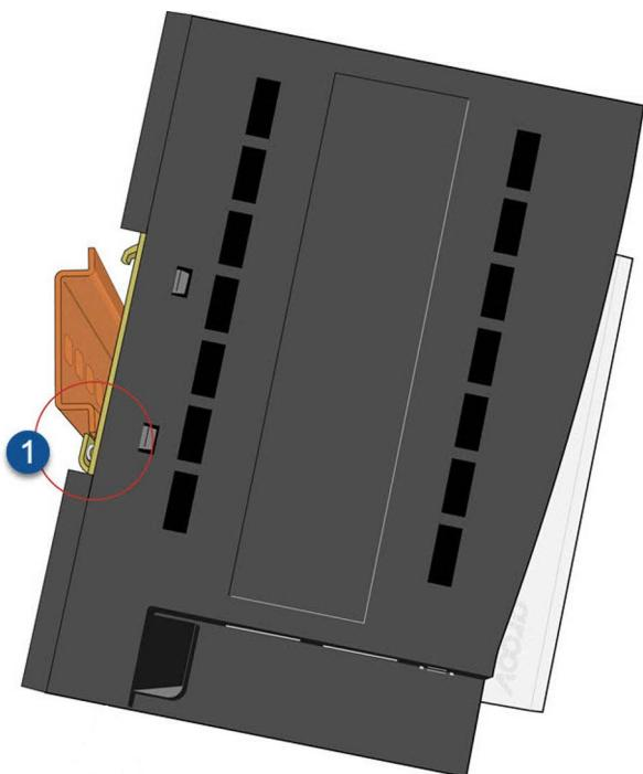
2. Push the bottom part of the module upward, making sure that you feel the clip catch on to the rail, and simultaneously push the top half of the module toward the DIN rail until the top of the DIN rail adapter engages the top lip of the DIN rail.
