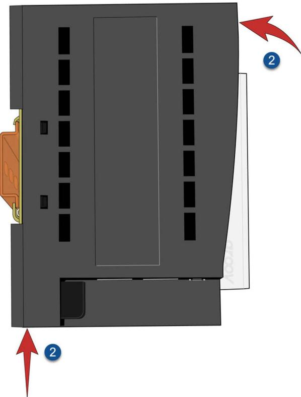
Before you release the module, verify that the top and bottom of the DIN rail adapters have engaged the DIN rail.
