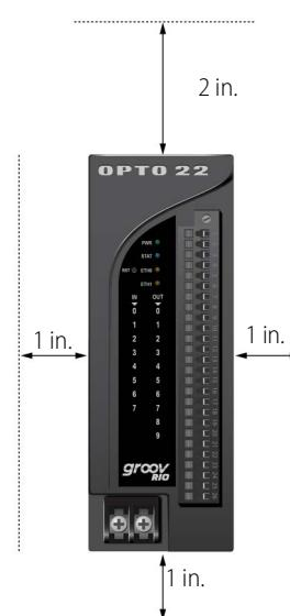
Make sure that there is a minimum of 2 inches clearance on the top, and 1 inch clearance on the bottom, each side, and in front of the *groov* RIO module, after it is mounted. Mount the module as shown in the diagram: with the Opto 22 logo at the top. Compliance with these guidelines helps ensure that the *groov* RIO module performs as described in the specifications.
