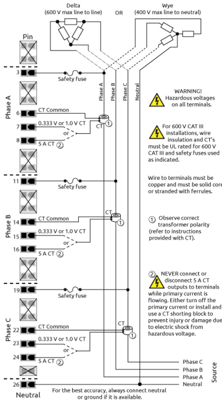
The following diagram illustrates how to correctly wire wye-configured loads when using potential transformers. Wye-configured loads over 400 V require potential transformers.
