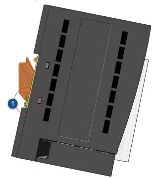
2. Push the bottom part of the module upward, making sure that you feel the clip catch on to the rail, and simultaneously push the top half of the module toward the DIN rail until the top of the DIN rail adapter engages the top lip of the DIN rail.
