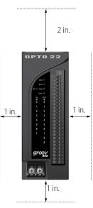
Make sure that there is a minimum of 2 inches clearance on the top, and 1 inch clearance on the bottom, each side, and in front of the *groov* RIO module, after it is mounted. Mount the module as shown in the diagram: with the Opto 22 logo at the top. Compliance with these guidelines helps ensure that the *groov* RIO module performs as described in the specifications.
