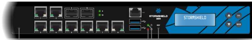
Reset to factory configuration button (defaultconfig)
