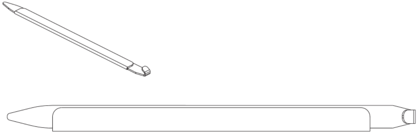
FIGURE 30 Optical transceiver extraction tool
