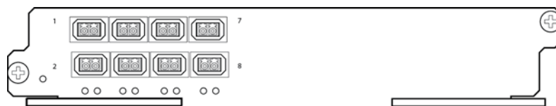
FIGURE 13 8x10GE-X module faceplate
