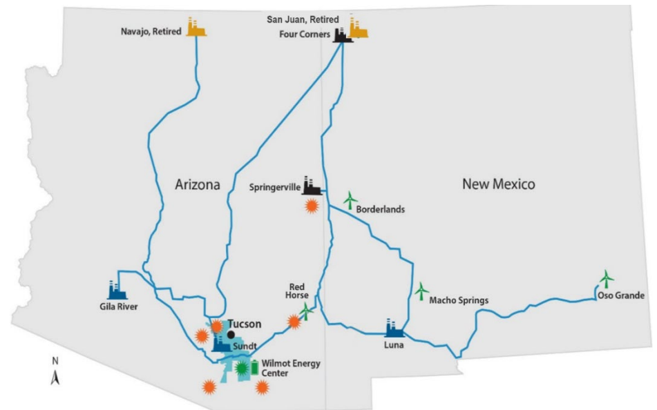
Figure 40. TEP Transmission and Generation Assets
