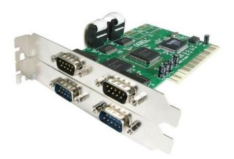
The PCI4S550N 4-port PCI Serial card turns an available PCI slot into four RS232 serial ports - a costeffective solution for connecting any new or old serial peripheral, with support for data transfer rates of up to 115Kbps.
