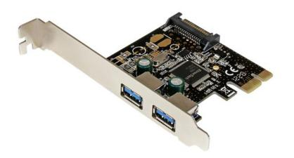
The PEXUSB3S23 2-Port PCI Express USB 3.0 Card lets you add two USB 3.0 ports to any PCI Expressenabled computer system. The USB card requires SATA power for functionality, and delivers 900mA of power per port to USB 3.0 bus-powered devices (500mA for USB 2.0) via your computers SATA power connector.
