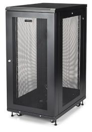
This server rack provides 24U of storage space in a sleek, secure cabinet for storing standard 19" rack-mount devices such as Dell, HP and IBM servers, along with telecommunication and A/V equipment. The rack is compatible with EIA-310 compliant equipment and supports a total load capacity of 450 kg (992 lb.).
