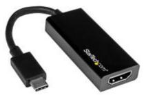
This USB-C<sup>™</sup> to HDMI® adapter lets you output HDMI video and audio from a USB Type-C<sup>™</sup> device such as a MacBook or Chromebook<sup>™</sup> laptop. This adapter works with USB-C devices that pass a DisplayPort video signal. It's also compatible with Thunderbolt<sup>™</sup> 3 ports.
