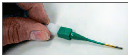
Plastic tool with contact in proper position.
