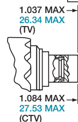
VIEW D FOR SIZE 8 TWINAX ONLY, RELATIVE TO -A-
