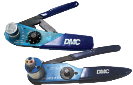
Examples of M22520 Series Crimping Tools:
