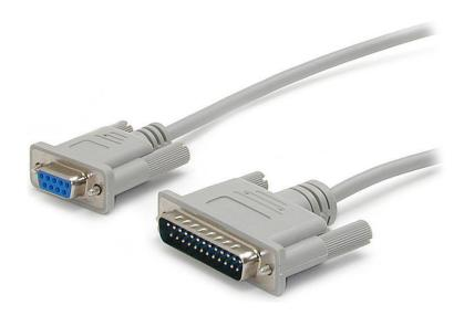
The SCNM925FM 10ft Cross Wired Serial/Null Modem Cable features one DB9 female and one DB25 male connector, allowing you to connect a 9-pin serial device to a 25-pin serial port, or transfer files from PC-to-PC via a serial connection.
