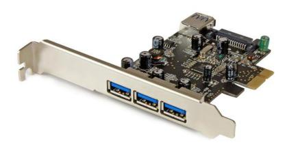
Here's a cost-effective solution for adding USB 3.0 connectivity to your computer. This 4-port PCIe USB 3.0 card gives you three external ports and one internal port, for the ultimate connection flexibility.
