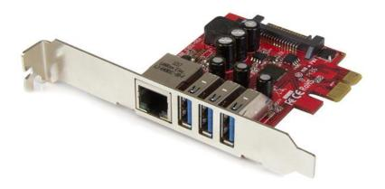
This PCIe USB 3.0 card couples your peripheral and network connections into a single, scalable solution.
