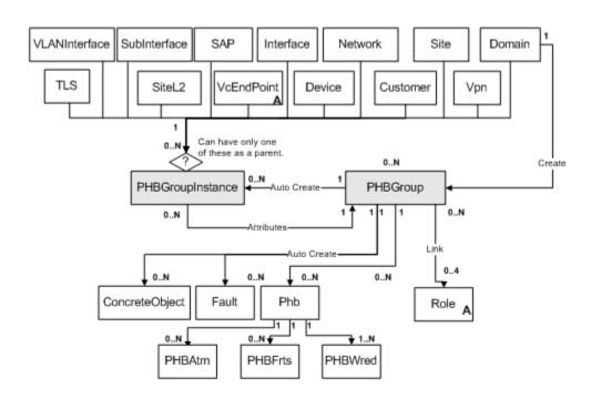
Figure 3-29 PHBGroup Object Diagram
