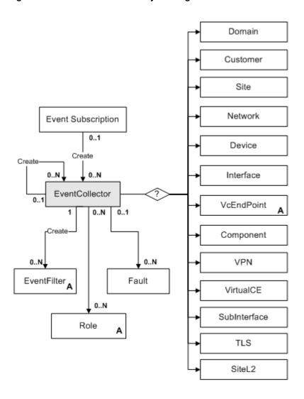
Figure 3-57 EventCollector Object Diagram
