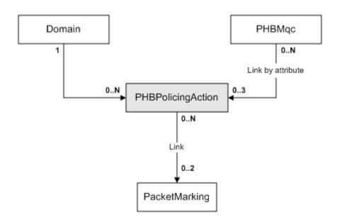
Figure 3-32 PHBPolicingAction Object Diagram
