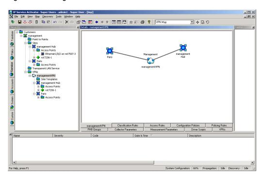
Figure 4-9 shows the properties box of the VPN, showing that "Management Site" is a hub, and "Paris" is a spoke.
