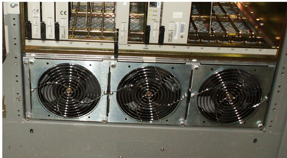
Figure 57: Fan tray inserted into fan tray bracket in the frame - front view
