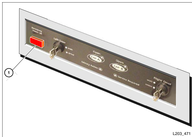
Figure 16. Emergency Robotic Stop Switch
