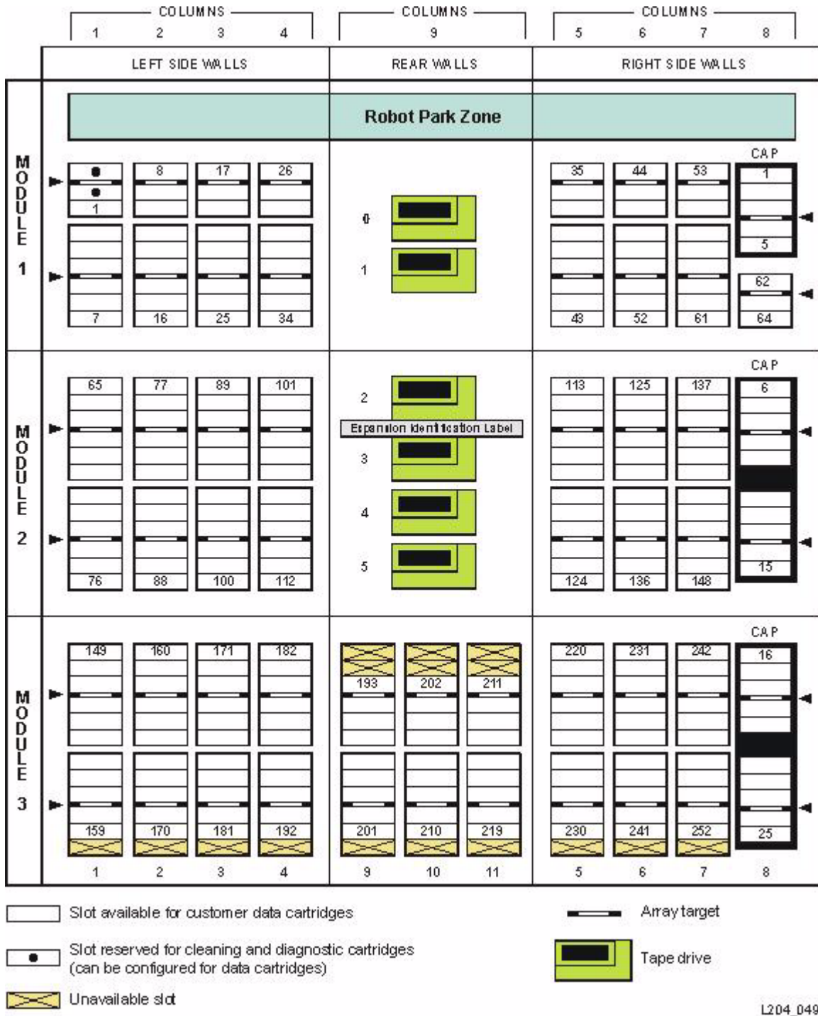
FIGURE 1-5 SCSI Element Numbering Mapping—LTO-only Library
