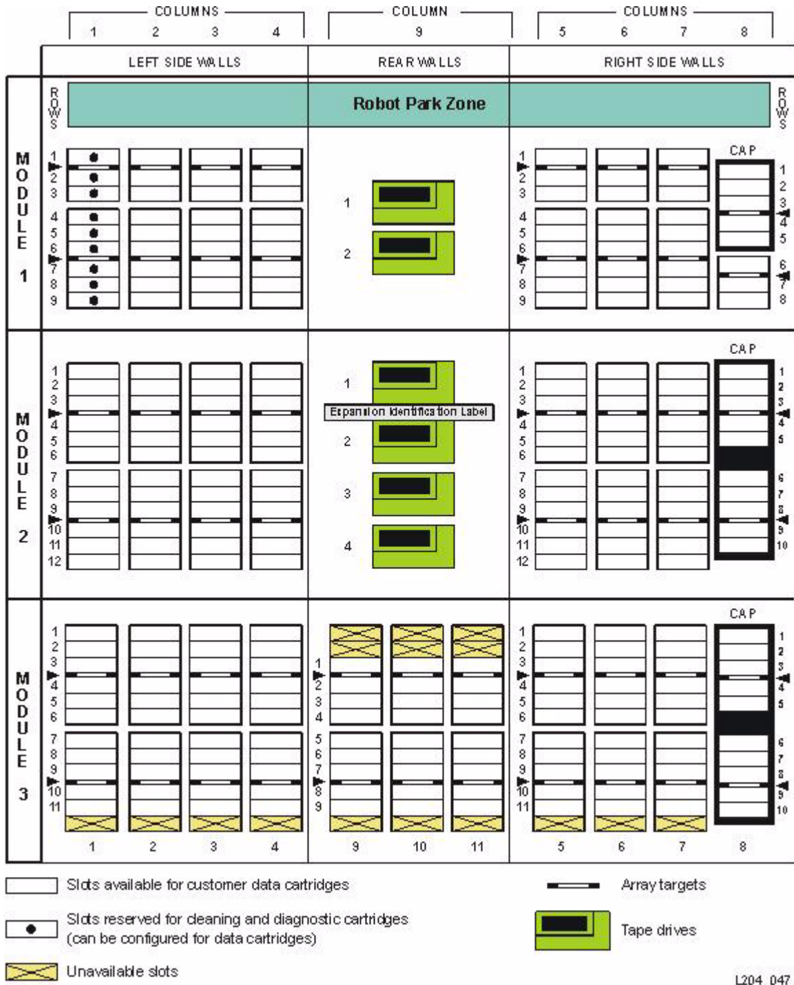
FIGURE 1-4 Firmware, LTO-only Library Slot Mapping
