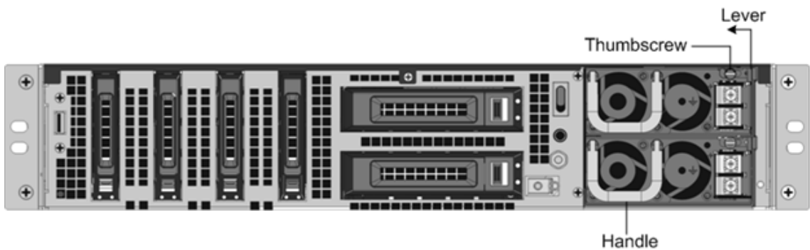
Figure 2. Remove an Existing DC Power Supply
