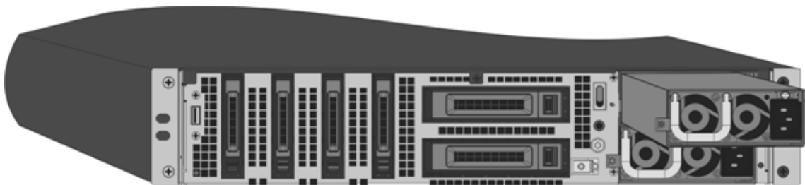
Figure 4. Insert the Replacement DC Power Supply
