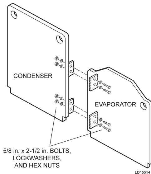
3. When the condenser and evaporator are both placed and bolted together, the supports should be removed for the final leveling process.
