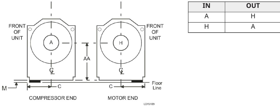
**Figure 46: Evaporators - compact waterboxes (2 pass nozzle arrangements)**
