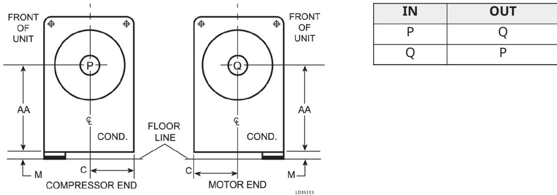
**Figure 50: Condensers - compact waterboxes (2 pass nozzle arrangements)**
