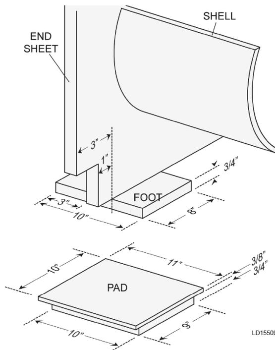
**Figure 28: Evaporator mounting on pad isolators**
