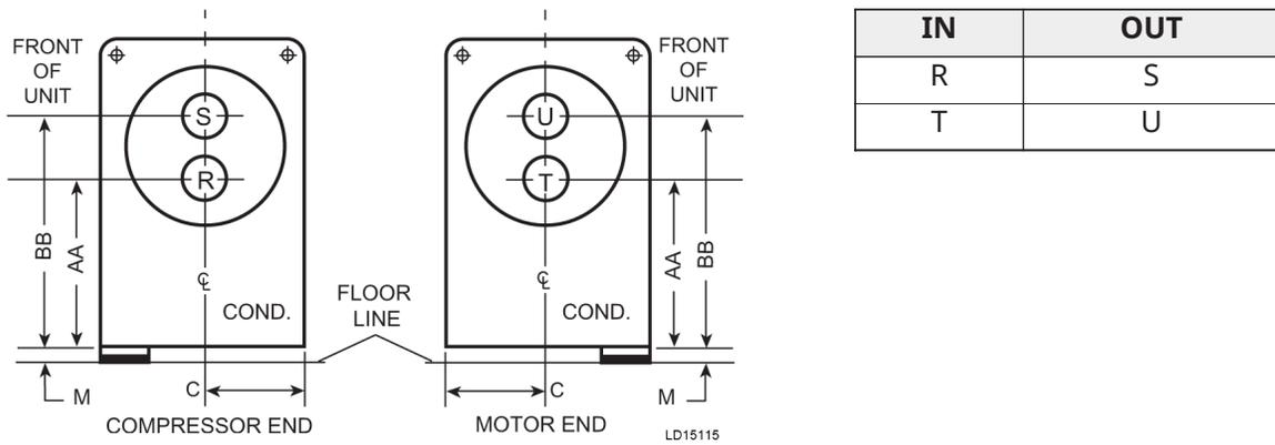
**Figure 51: Condensers - compact waterboxes (3 pass nozzle arrangements)**
