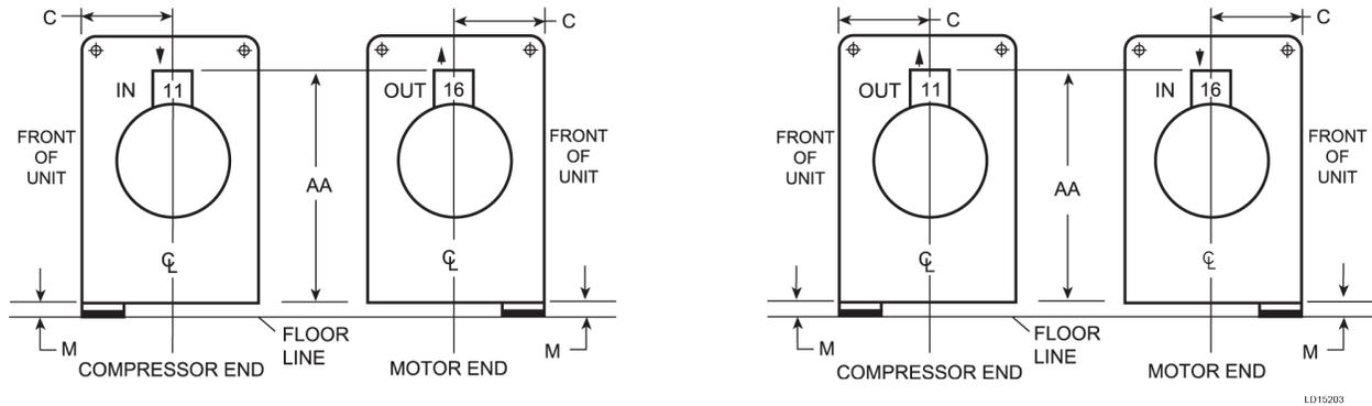
**Figure 58: Condensers - marine waterboxes (2-pass nozzle arrangements)**
