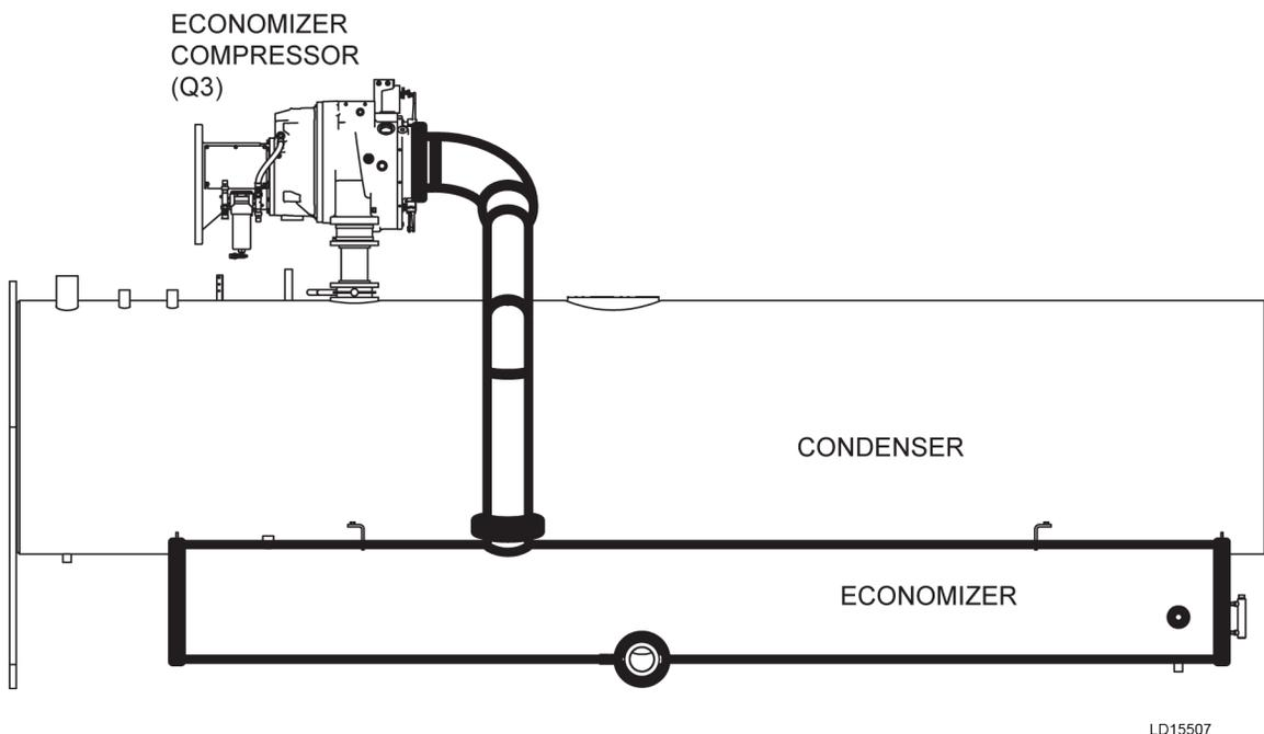
**Figure 25: Insulating the economizer and economizer suction pipe (front view)**
