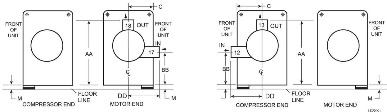
**Figure 59: Condensers - marine waterboxes (3-pass nozzle arrangements)**
