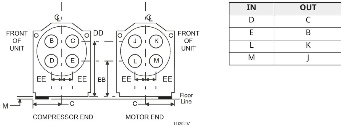
**Figure 47: Evaporators - compact waterboxes (3 pass nozzle arrangements)**
