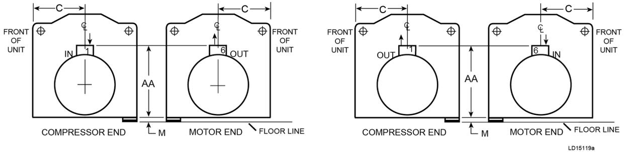
**Figure 54: Evaporators - marine waterboxes (2-pass nozzle arrangements)**
