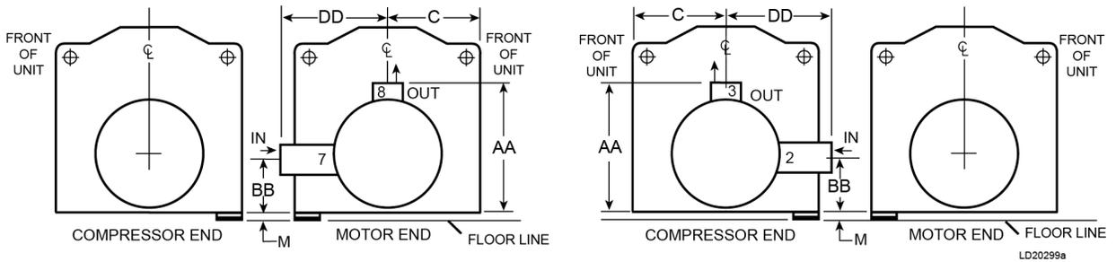
**Figure 55: Evaporators - marine waterboxes (3-pass nozzle arrangements)**
