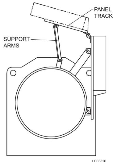
2. Swing the control center into a vertical position. See [Figure 42](#).
