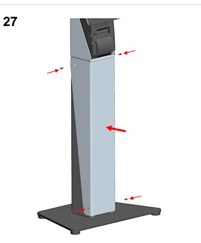
Replace floor stand cover and secure using (4) screws saved from step 2.
