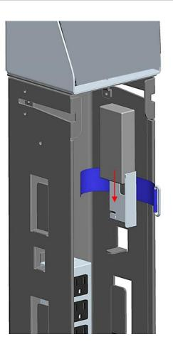
Add power bricks into tower using provided straps.
