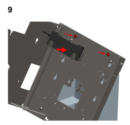
Assemble USB Hub. Add (2) screws from bag "S"; leave ~3mm (1/8") gap for USB bracket to slide on; tighten screws.
