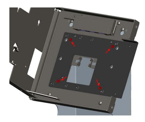
Remove Fill Plate on Display Bracket.
