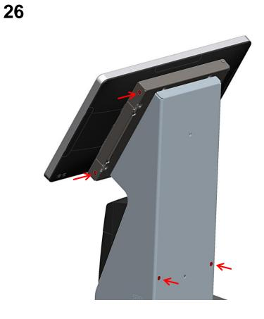
Close Display Bracket and add (2) screws saved from step 7. Secure printer assembly with (2) screws saved from step 3.
