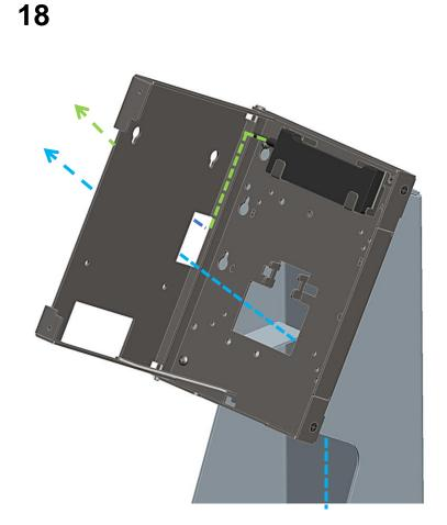
Before attaching i-Series, route **power**, **LAN cables** through bottom of stand head and through Display Bracket. Route **USB Hub** cable or other **USB** if used.
