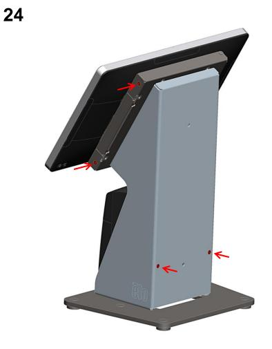
Close Display Bracket and add (2) screws saved from step 5. Secure printer assembly with (2) screws saved from step 1. If installing an EMV Cradle, finish by adding (1) screw from bag "N".
