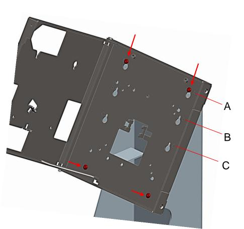
Assemble Display Bracket onto Head. Position "A" for 15", 22" in landscape. Position "B" for 15" in portrait Position "C" for 22" in portrait Add (2) screws from bag "A" at bottom holes.
