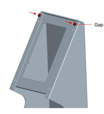
Add (2) screws from bag "A"; leave ~3mm (1/8") gap (for Display Bracket).
