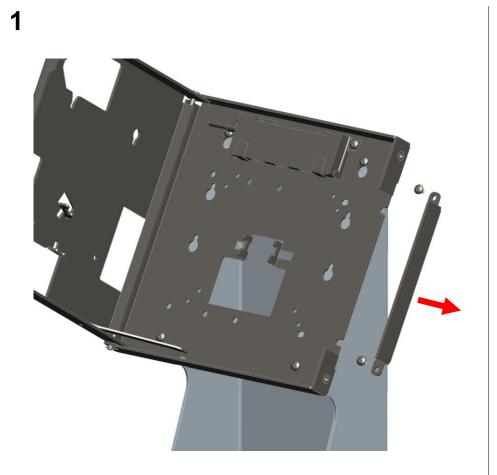
Remove Fill Plate on Display Bracket.
