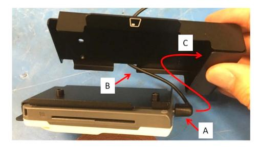
Add USB cable to RP757 (A), insert RP757 + sled into sled bracket (C) shown. Make sure cable exits through slot (B) when assembled.
