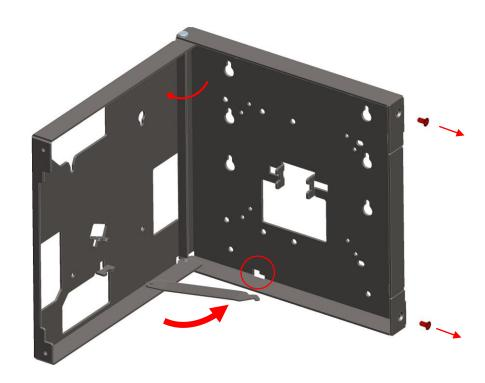
Remove and save (2) screws, open cover of Display Bracket; pivot out and fix prop.
