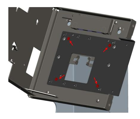
Add the EMV Mount Plate to the Display Bracket using (4) screws from bag "R".
