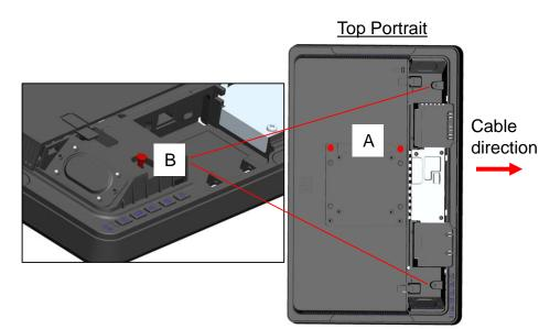
Add (2) screws from bag "T" at positions labeled "B". Leave ~3mm (1/8") gap for later mounting of Cable Bracket.
