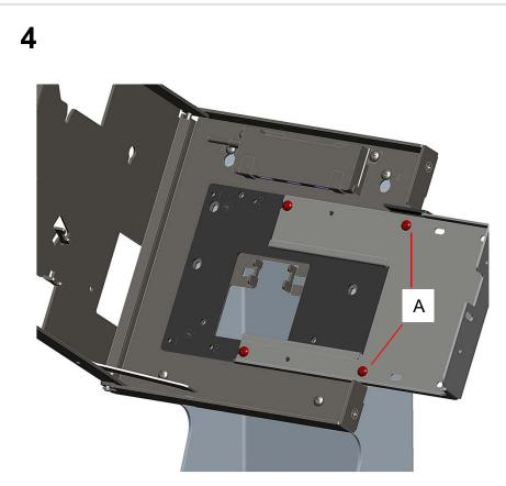
Assemble EMV Arm to Display Bracket. Add (2) screws from bag "P" at right most position "A" to secure EMV Arm to Display Bracket.
