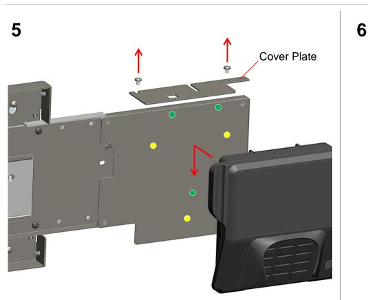
Remove and save EMV Cover Plate and screws. Add (3) screws for mounting EMV terminal:
