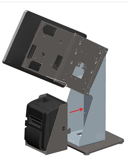
Route cables from/to printer as needed, slide in printer tray assembly (or printer tray with cover if no printer).
