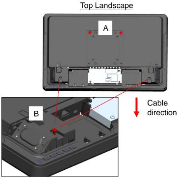
Add (2) screws from bag "T" at positions labeled "B". Leave ~3mm (1/8") gap for later mounting of Cable Bracket. Add tie-wrap
