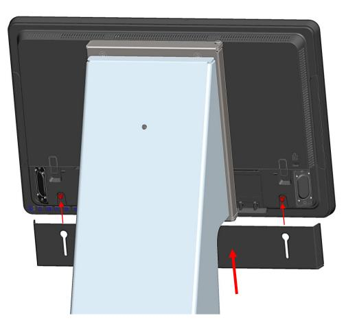
Attach metal Cable Cover and tighten (2) screws.
