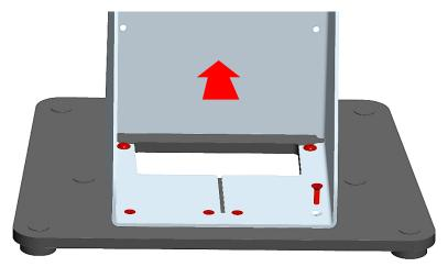
Align slots on bottom rear of Head with (2) screws on base and slide on stand. Add (4) screws from bag "B". Tighten (2) previous screws at rear.
