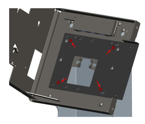
Remove Fill Plate on Display Bracket.
