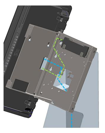
Close Display Bracket and attach cables to i-Series. Attach metal Cable Cover and tighten (2) screws. Open Display Bracket, rout and tie-wrap cables.
