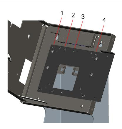
Add (2) screws to EMV Mount Plate from bag "P" at position 1, 2,3 or 4. Leave ~3mm (1/8") gap (for EMV Arm).
