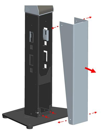
Remove and save the (4) screws on the left and right of the stand front cover. Pull off the silver cover and set aside. Add (2) remaining screws from bag "K" to bottom front of stand.
