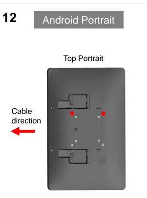
Add (2) screws from bag "L" to top VESA positions. Leave ~3mm (1/8") gap for mounting to display bracket. Remove cable cover(s) before mounting displays on stand.
