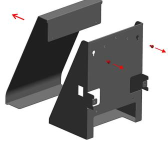
If using printer, remove cover to add printer.
