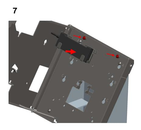
Assemble USB Hub. Add (2) screws from bag "S"; leave ~3mm (1/8") gap for USB bracket to slide on; tighten screws.
