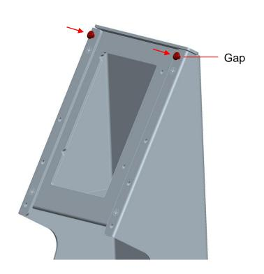
Add (2) screws from bag "A"; leave ~3mm (1/8") gap (for Display Bracket).
