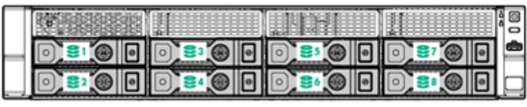
8-bay LFF hot-plug drive model
