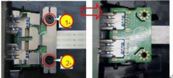
Use a Philips-head screwdriver to remove 2 screws for unlocking USB board.
