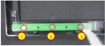
Use a Philips-head screwdriver to screw 3 screws for locking key board (No.1~3 screw size=M2x2.5; Torque=0.9±0.4kgf.cm
