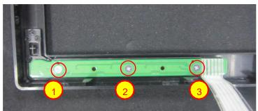
Use a Philips-head screwdriver to remove 3 screws for unlocking key board
