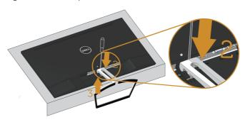
**4.** While pressing on the release button, pull the stand out.
