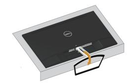
**3.** Use a long screwdriver to press on the release button.
