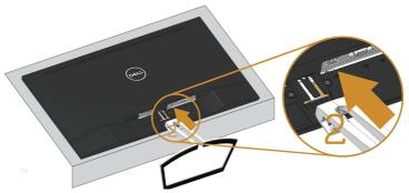
3. Inserting the stand until the snap lock.
