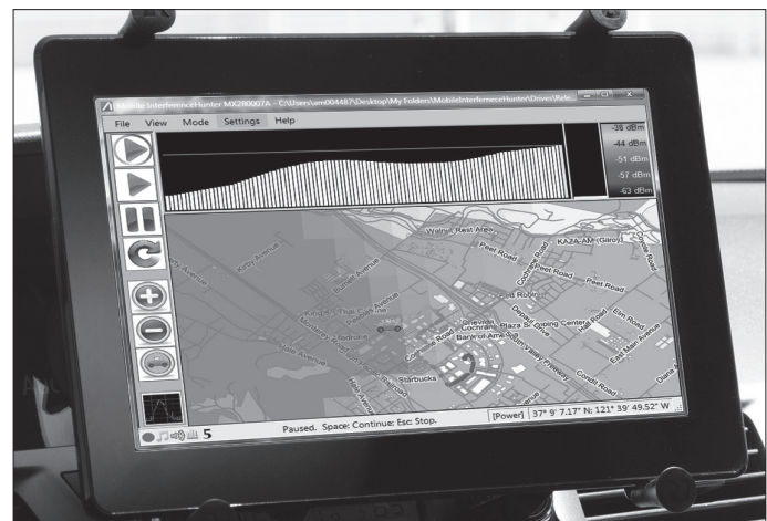
OpenStreetMap™ displayed on Windows PC tablet. Interference hunt screen capture. Dots shown along drive path are colored according to signal strength.
