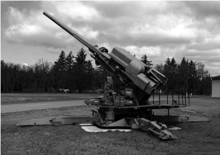
5.4 120-mm anti-aircraft gun, deployed near the end of World War II. These guns were automatically aimed using negative feedback by the M10 director system, which used information from a radar system, and the M4 gun computer. This gun is on display at the Washington National Guard Museum, located on Camp Murray in Washington State. Courtesy of the Washington National Guard State Historical Society.
