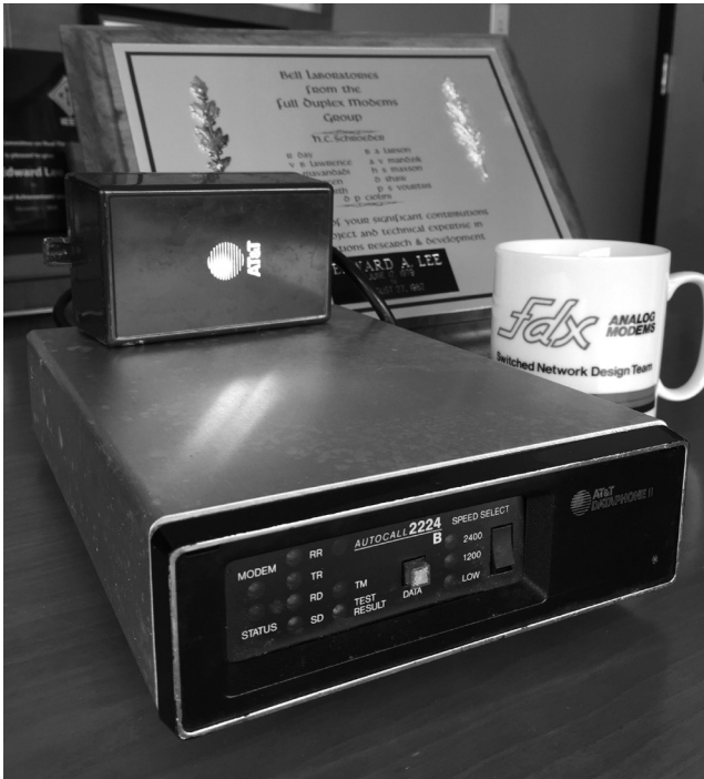
9.1 A vintage voiceband data modem, the first to be realized by software, designed by the author and colleagues at Bell Labs in the early 1980s.
