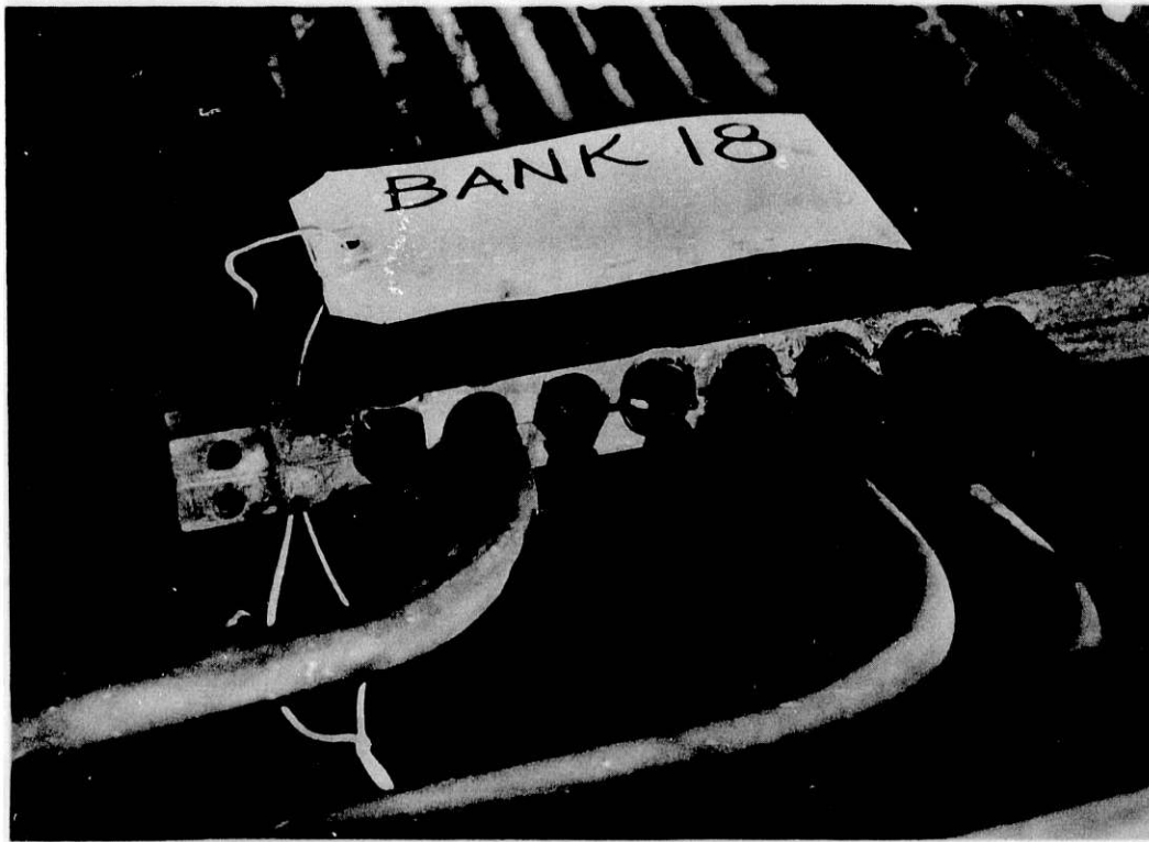
Fig. 1.1. Steam Generator Tube Bank Damaged by Vibration (Shin and Wambsganss 1977) (ANL Neg. Nos. 113-84- 88 and 113-84-89)
