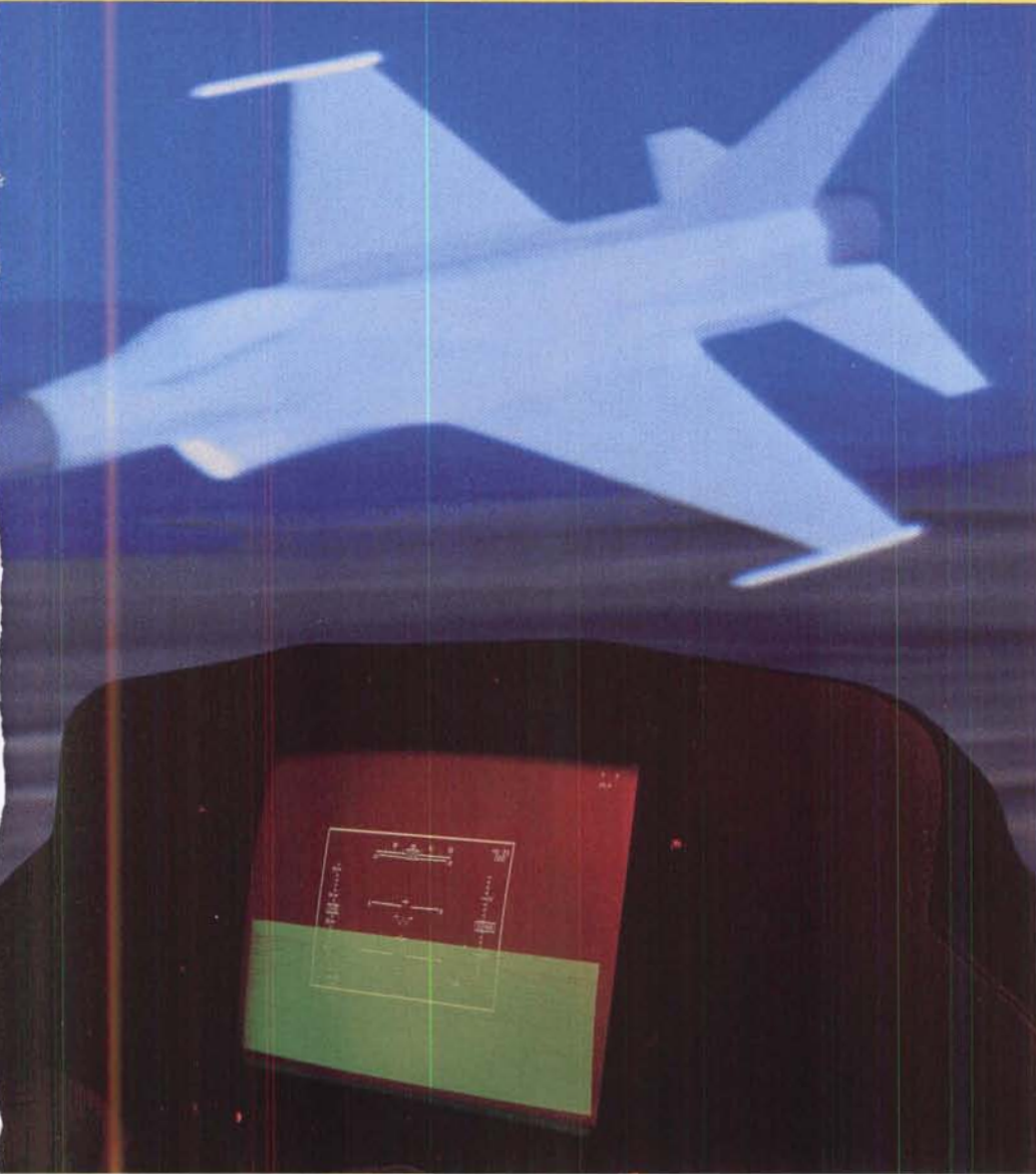
Within the MS-1, laser projectors used to create the image of other aircraft are mounted fore and aft of the simulation cockpit.
