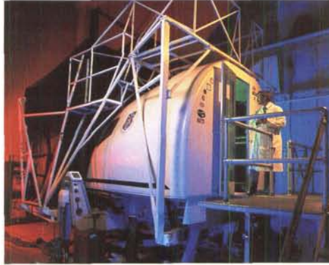
The KC-135 cab and the F-111 cockpits provide two-man, side-by-side simulation capability. These reconfigurable simulators allow for unique vehicle simulations and aircrew interaction studies.
