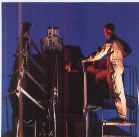
Within the MS-1, laser projectors used to create the image of other aircraft are mounted fore and aft of the simulation cockpit.
