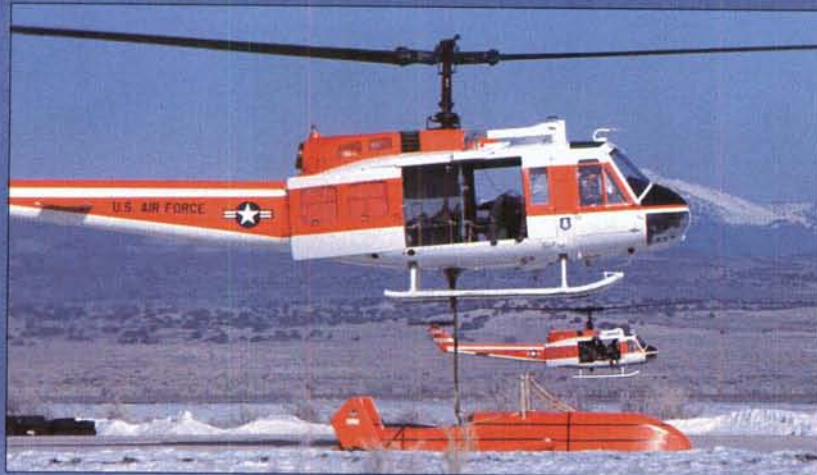
Helicopter airlifting UAV to Recovery Area
