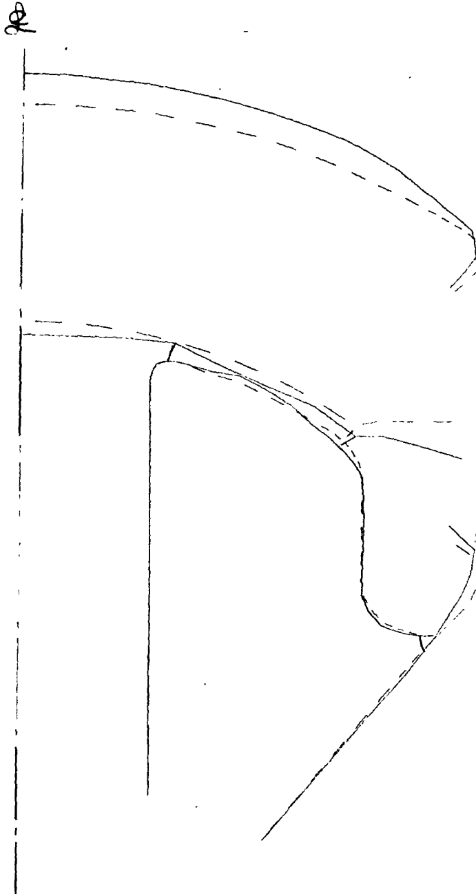
Fig. 2. Deformed Geometry of Accumulator under max pressures
