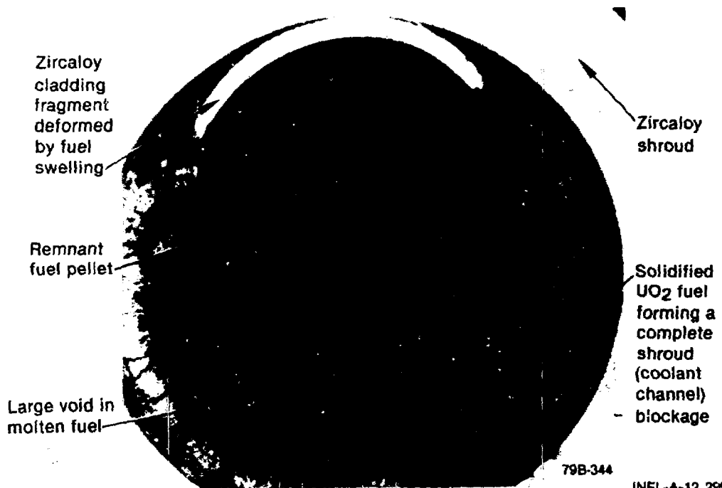
Figure 2. Ground and polished cross section of Rod 801-1 showing fuel, cladding, and shroud near the peak power elevation (Test RIA 1-1).
