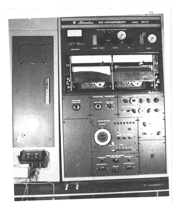
FIGURE 2 Photograph of the gas chromatograph.
