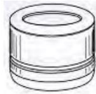
TYPE 1 (SNAP RING GROOVES IN BEARINGS)
